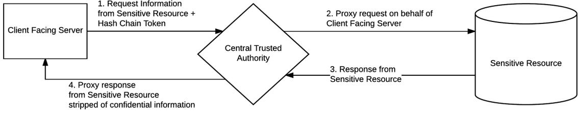
Figure 1: Architectural overview of the system. This figure describes the three primary modules involved. The client facing server, The central trusted authority and a sensitive resource.
