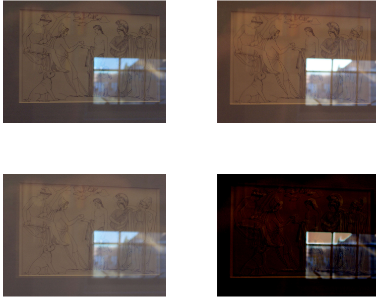
FIGURE 10. The Judgement of Paris by Flaxman with a reflection of my window which overlooks Drumheller Fountain. In the top row are the two original photos taken with linear polarizer rotated 90 degrees between shots. The bottom row represents the separated images. The brightness of the reflected image greatly effects the quality of the image separation.
