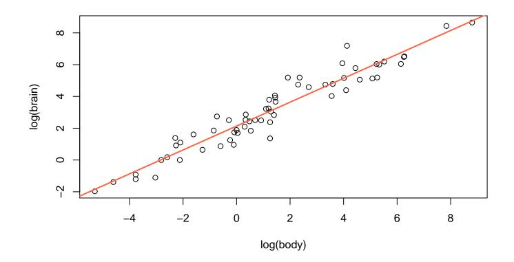
Straight line suggests log(brain) higher by  $\approx 0.75$  units, per 1-unit difference in log(body) – i.e. a power law, brain  $\propto$  body<sup>0.75</sup>.
