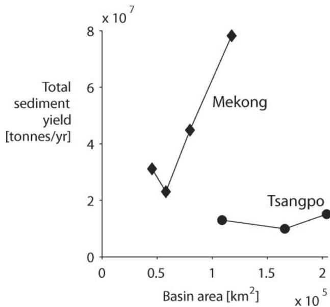
**Figure 7.** Cumulative sediment yield as a function of upstream area. The slope of the line is the erosion rate between two points. It is apparent from this figure that the upper Tsangpo River has a much lower overall erosion rate than the Mekong River.
