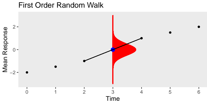
Figure 8: Illustration of the RW1 model for smoothing at time 3. The mean of the smoother is the average of the two adjacent points (and is highlighted as ●), and deviations from this mean are penalized via the normal distribution shown in red.
