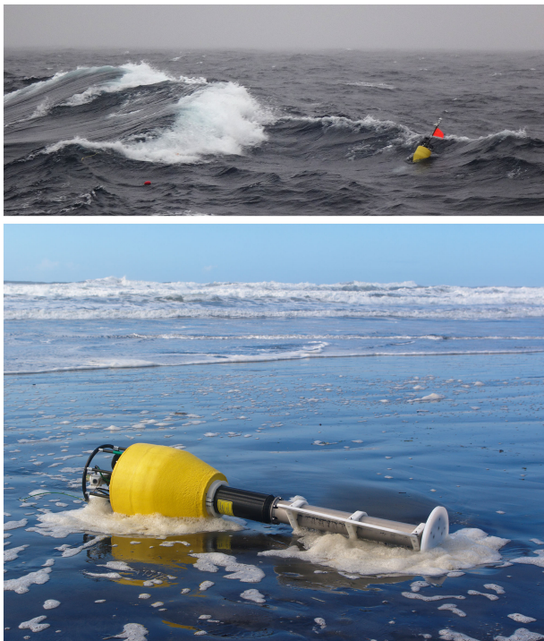
Fig. 2. Top: A SWIFT is impacted by a small breaking crest as a larger breaking wave approaches. Bottom: A SWIFT on the beach after drifting back to shore.
