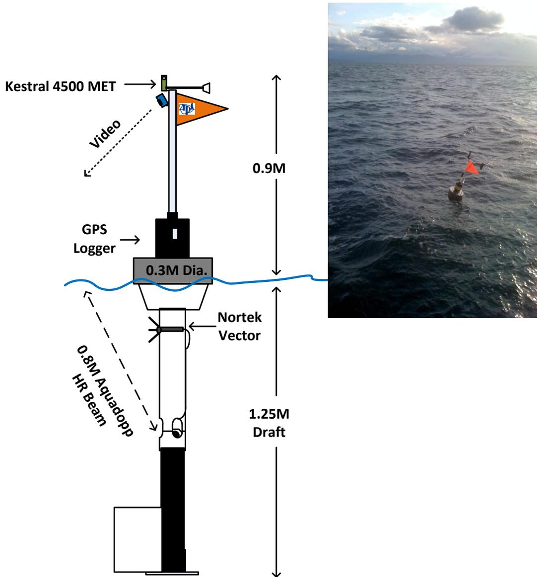
FIG. 1. (a) Dimensional drawing and (b) picture of a SWIFT: Surface Wave Instrument Float with Tracking. Drawing and design by J. Talbert, APL-UW.
