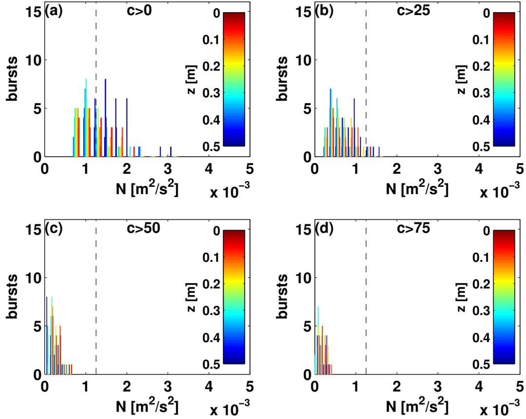
FIG. 10. Distributions of noise intercepts  $N$  from all bursts at Duck FRF using four different pulse correlation  $c$  cutoffs for quality control of velocity data. (a) is  $c > 0$ , (b) is  $c > 25$ , (c) is  $c > 50$ , and (d) is  $c > 75$ . Colors indicate distance beneath the wave following surface, as in Figure 6. Dashed lines indicate the predicted value for  $N$ , given a Doppler velocity uncertainty of  $\sigma_u = 0.025$  m/s.
