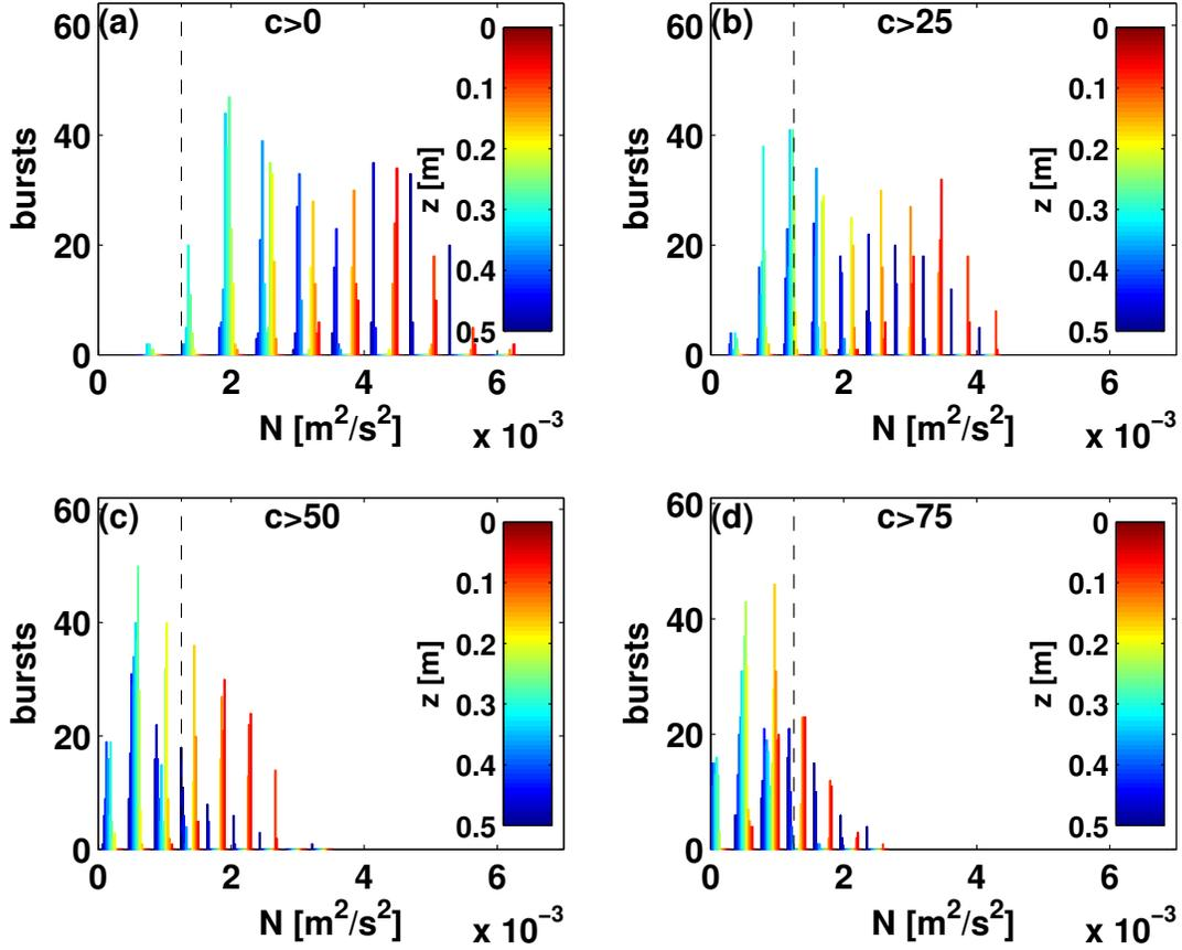
FIG. 11. Distributions of noise intercepts  $N$  from all bursts on Lake WA using four different pulse correlation cutoffs for quality control of velocity data. (a) is  $c > 0$ , (b) is  $c > 25$ , (c) is  $c > 50$ , and (d) is  $c > 75$ . Colors indicate distance beneath the wave following surface, as in Figure 7. Dashed lines indicate the expected range for  $N$ , given a Doppler velocity uncertainty of  $\sigma_u = 0.025$  m/s.
