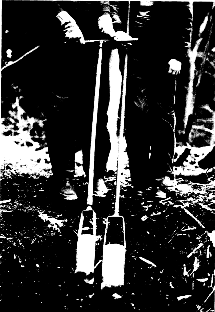
Figure 1. These two manual bucket augers have 4-inch buckets and extension rods of two different lengths. The bucket auger is used by placing the screw-type bit on the surface and rotating downward. The bit digs into the substrate while the sediment is pushed into the bucket. The helical motion and the action of the bit disturbs the context of the sediment. When the bucket is full the auger is brought to the surface and the contents emptied. The auger is then lowered back into the hole, repeating the whole process until the bucket is full again. The handle and extension rod can be removed from the auger head to allow additional rods to be added and greater depths reached. However, I found that having two augers, attached to a short and a long rod, eliminates the difficult process of unscrewing the rod from the head. When a depth equal to the length of the short auger is reached, the other auger is used. (Photo taken by the author at 45-SJ-24, San Juan Island National Historic Park-British Camp.)
