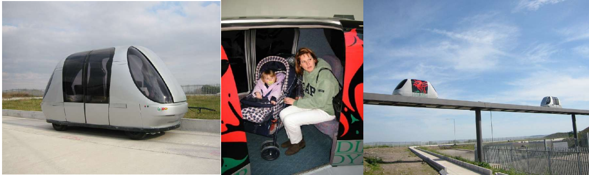
Fig.3: ULTra vehicle by the Advanced Transit Systems Ltd, UK. Left: Vehicle running on ground-level. Center: On-level boarding with stroller. Right: Two vehicles on elevated guideway.
