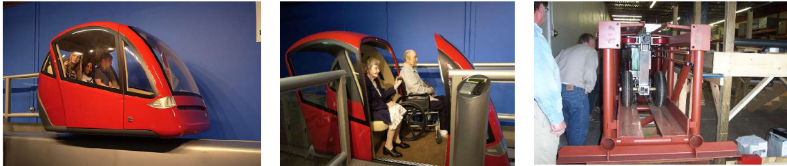
Fig.4: Prototype of Skyweb Express by the Taxi2000 Inc, USA. Left: Vehicle on short test track. Center: Open vehicle with wheelchair passenger at station. Right: Vehicle chassis inside guideway which has a cross section of approximately 1m by 1m.
