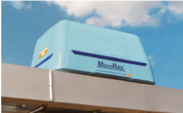
Automated MicroRail cargo cars carry up to 1,000 lbs of cargo on guideways at 65-mph
