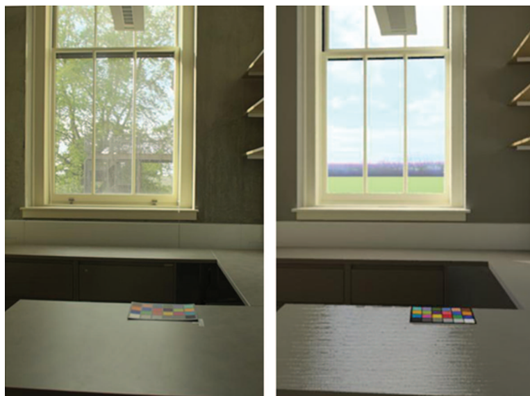
Fig. 12. Photograph and simulated image of the office under partly cloudy sky.
