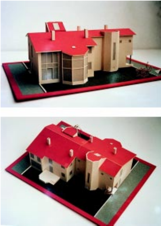
Fig. 2. Model of the conventionally designed and the energy consciously designed dwellings.
