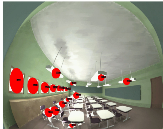
Fig. 9 Fisheye view of the classroom with glare analysis (Radiance)
