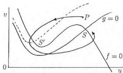
**Figure 6.10.** Reaction kinetics null clines which illustrate a threshold behaviour. With a perturbation to  $P$ , the solution embarks on a large excursion in the phase space before returning to the stable steady state  $S$ . A similar threshold behaviour is possible if the null clines intersect at the steady state  $S'$ .
