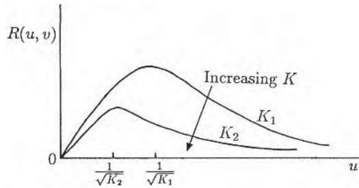
**Figure 6.7.** Reaction rate  $R(u, v)$  in (6.117) for a fixed  $v$ . The reduction in  $R$  as  $u$  increases for  $u > 1/\sqrt{K}$  is a typical example of substrate ( $u$ ) inhibition: the larger the  $K$  the greater the inhibition.
