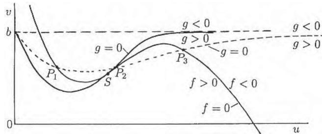
**Figure 6.8.** Schematic null clines for the substrate–inhibition kinetics (6.117). There may be one,  $S$ , or three,  $P_1, P_2, P_3$  (dashed  $g = 0$  curve) steady states where  $f = 0$  and  $g = 0$  intersect. Note the signs of  $f$  and  $g$  on either side of their null clines.
