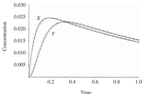
**Figure 6.4.** Case 2 composite (---) solutions compared to numerical solutions (—) for  $X$  and  $Y$ , the intermediate concentrations. Parameters are the same as in Figure 6.3. (From Burke et al. 1990)
