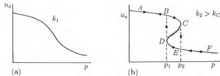
**Figure 6.11.** (a) Typical variation of the steady state  $u_s$  as a function of a parameter  $p$  in the kinetics for a fixed value  $k_1$  of another kinetics parameter  $k$ . (b) As the parameter  $k$  passes through a bifurcation value  $k_c$ , multiple steady states are possible when  $p_1 < p < p_2$ . The steady state that lies on the branch  $DC$  is unstable.
