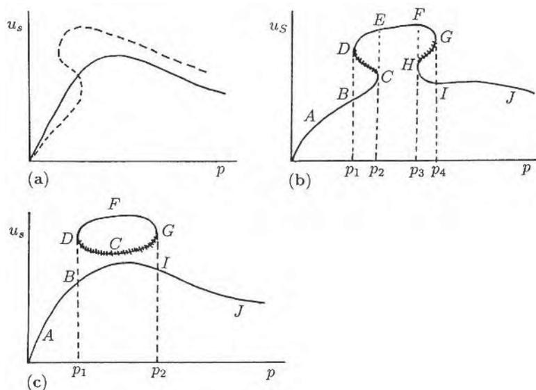
**Figure 6.12.** (a) Another typical example of a steady state dependence on a parameter with transition to multiple steady states; compare with Figure 6.11 (a). (b) Typical mushroom dependence of the steady state as a function of a parameter  $p$ . (c) This shows an example of an isola: it can be a natural evolution from the form in (b).
