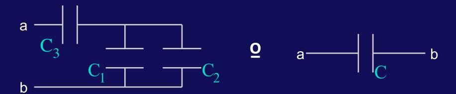
Note: C<sub>3</sub> is in series with the parallel combination on  $C_1$  and  $C_2$ . *i.e.*
