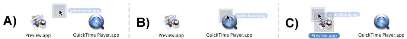
Figure 3. Illustration of how MacOSX indicates drag-drop applicability (Microsoft Windows has a similar behavior). A) The user begins to drag a JPG document. B) User drags the file over the QuickTime Player application. There is no highlight because QuickTime is not able to open JPG files. C) User drags the file over the Preview application. This application can open JPG files; the blue highlight indicates the file can be “dropped” here.
