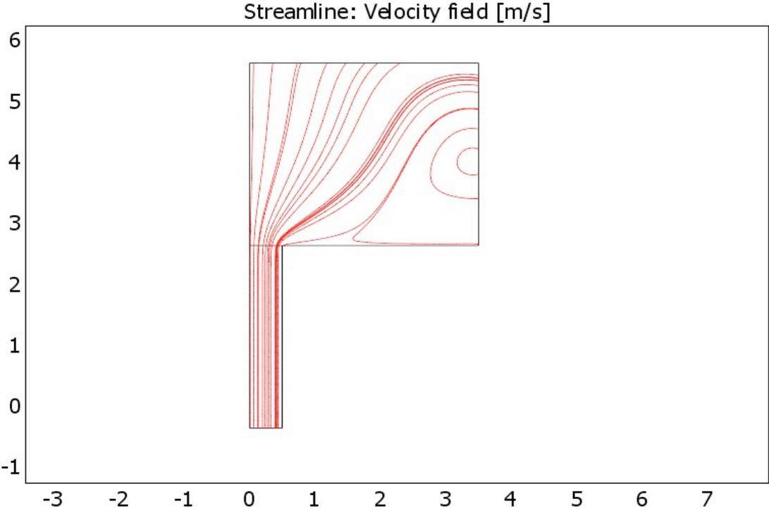
Figure 8 . Sharp edged exit (Re=0)
