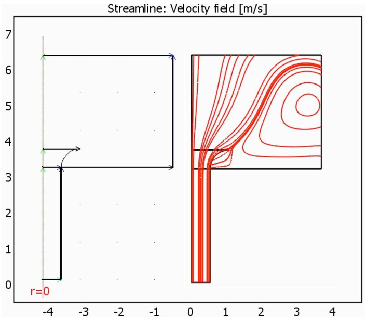
Figure 11. Bellmouth Streamline profile at  $Re=0$
