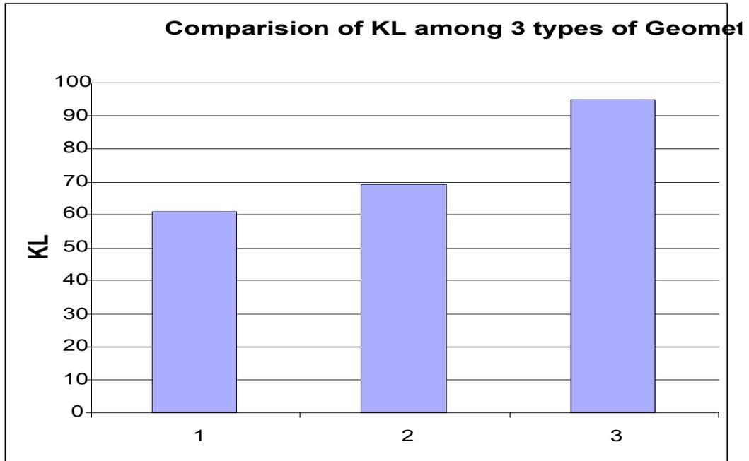
Figure 4. Comparison of KL for Well round, projecting, and sharp edge models ( $Re=0$ )
