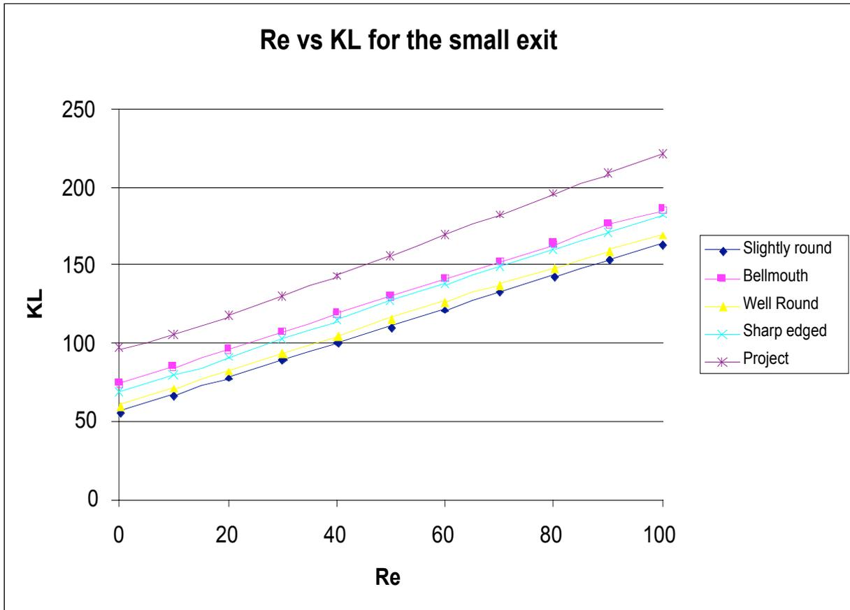
Figure 7. Comparison of KL among 5 shapes at different Reynolds numbers.
