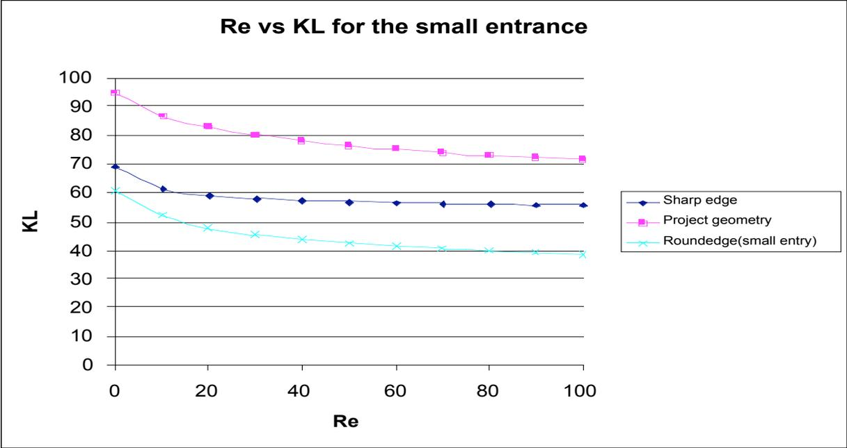
Figure 6. Comparison of KL among 3 shapes at different Reynolds numbers
