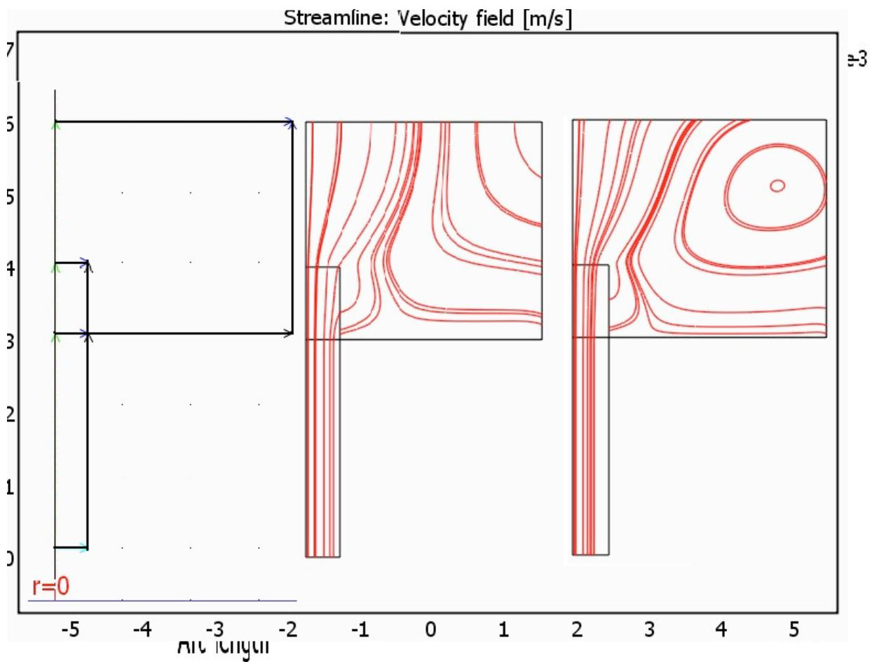
Figure 13 . Projecting pipe exit, projecting pipe entrance
