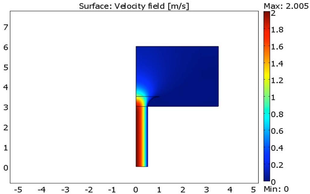
Figure 3. Bellmouth Model with velocity profile
