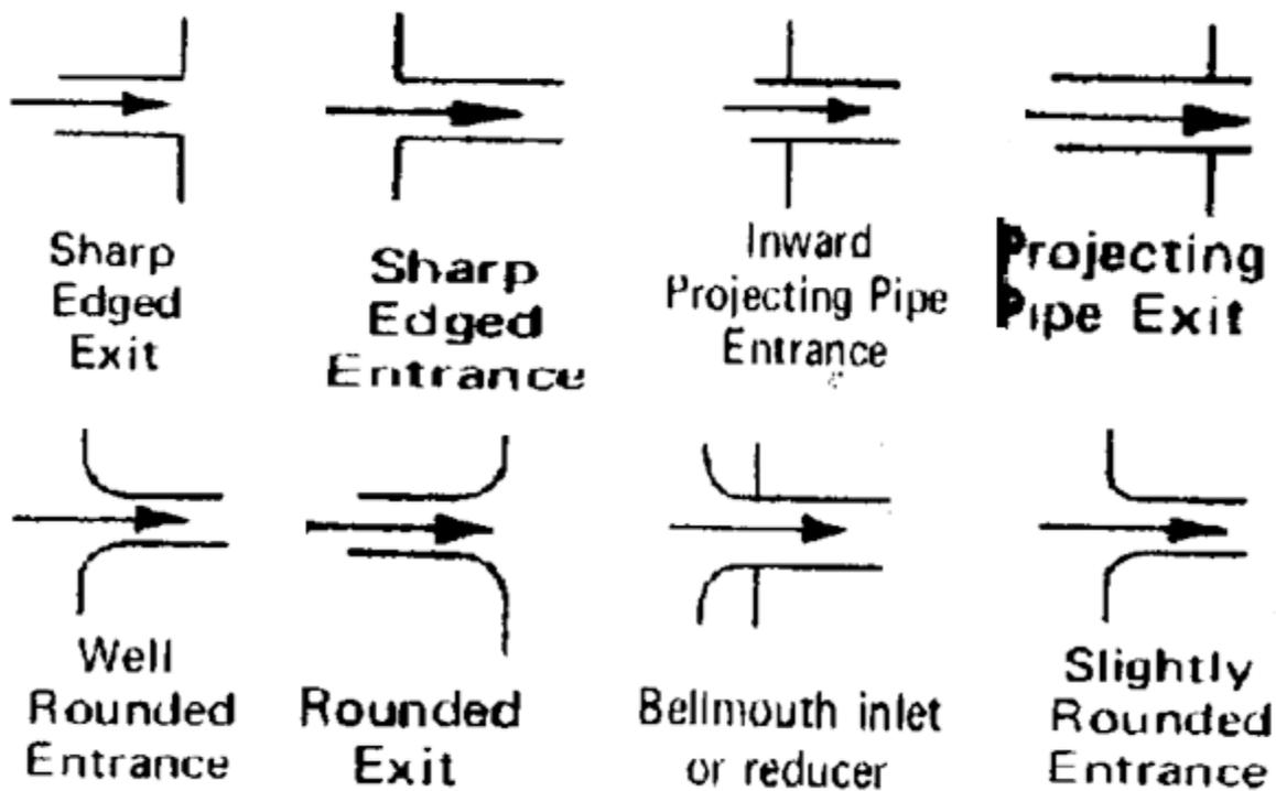
Figure 1. Eight models: Different Geometries in microfluidic devices
