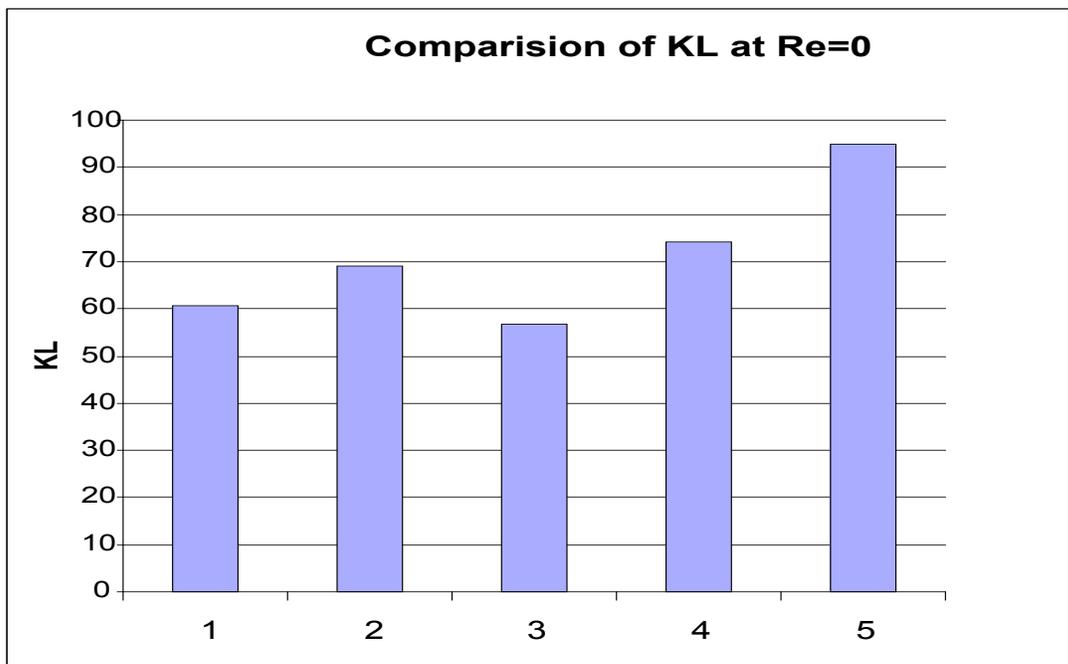
Figure 5. Comparison KL for well round, projecting, bellmouth, slightly round, sharp edged models ( $Re=0$ )
