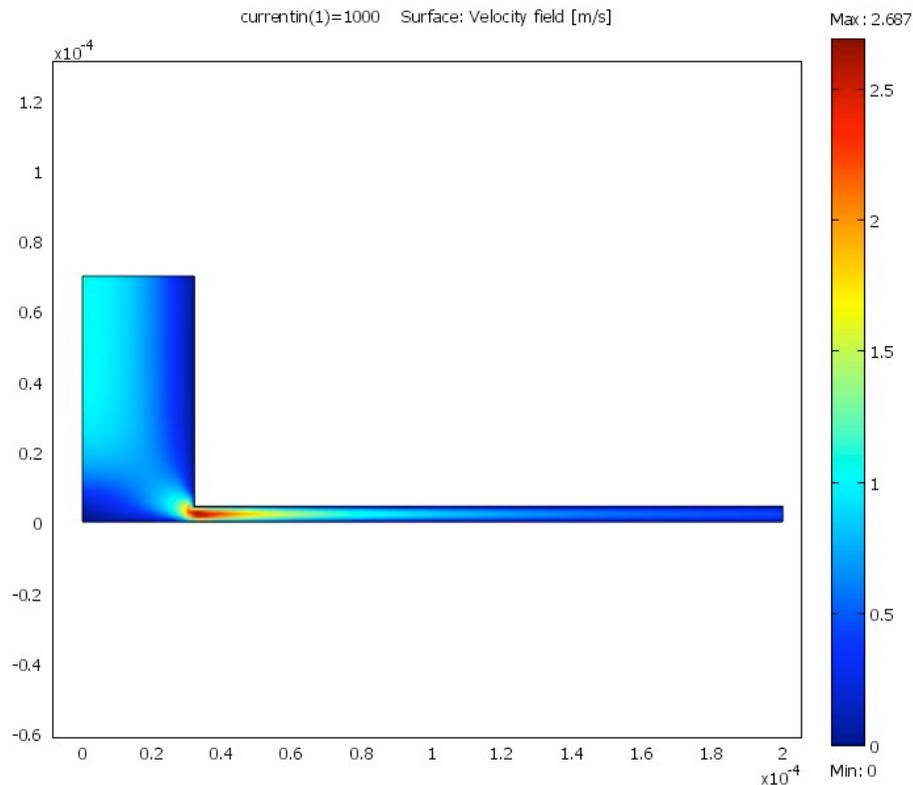
Figure 3: Surface Plot of Velocity Field obtained from Navier Stokes Analysis
