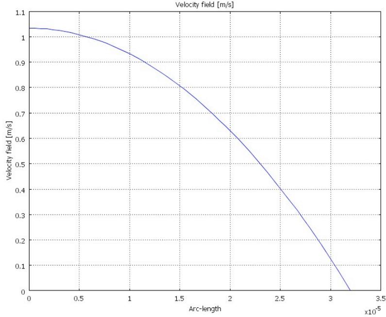
**Figure 4: Radial Velocity Distribution in Nozzle**
