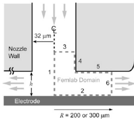
Figure 1: Geometry used to model EcP <sup>[1]</sup>
