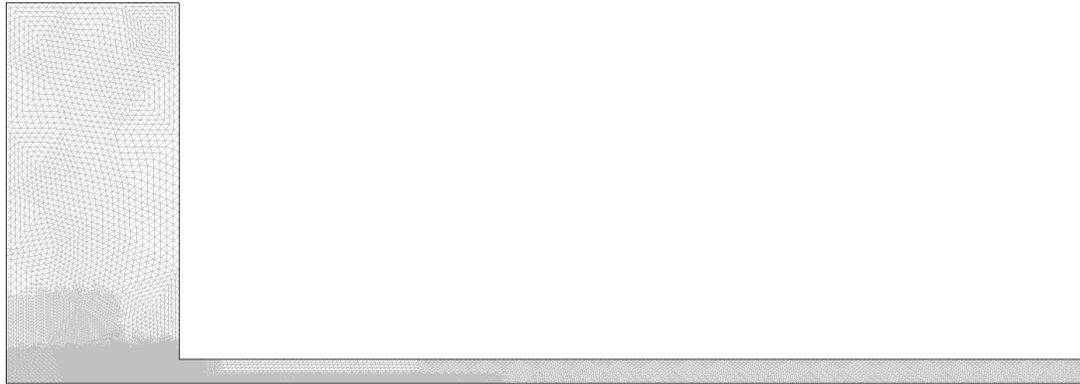
**Figure 5: Refined mesh applied to model before solving Nernst Planck Physics**
