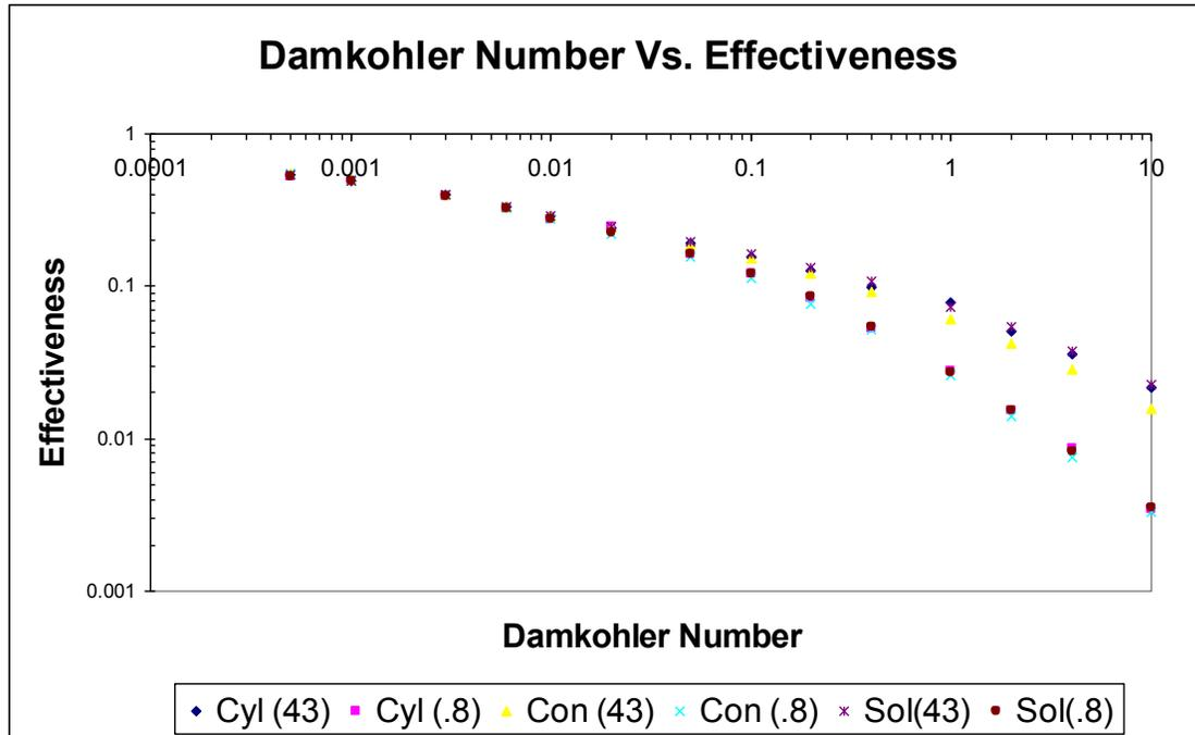
Figure 6: Plot of the Damkohler number versus the Effectiveness on a log-log scale. The legend at the bottom describes the geometry and diffusivity ratio that is represented within the graph.
