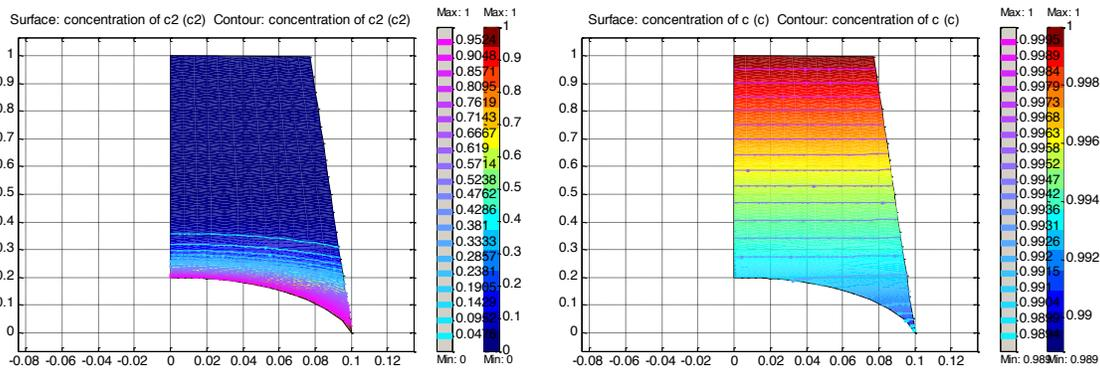
Figure 13 and 14: Concentration Profiles for Oxygen ( $c_2$ ) and the Electrolyte ( $c$ ) for a Diffusivity Ratio = 43, Damkohler Number = 0.1
