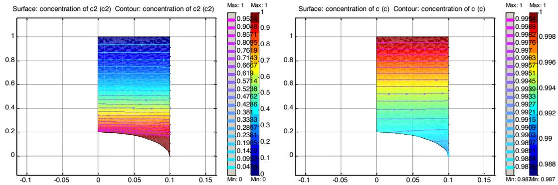
Figure 7 and 8: Concentration Profiles for Oxygen (c2) and the Electrolyte (c) for a Diffusivity Ratio = 0.8, Damkohler Number = 0.001
