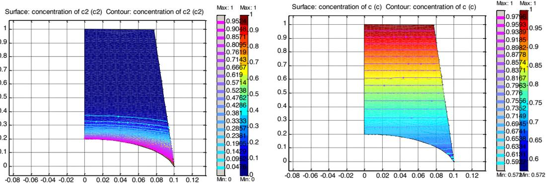
Figure 11 and 12: Concentration Profiles for Oxygen ( $c_2$ ) and the Electrolyte ( $c$ ) for a Diffusivity Ratio = 0.8, Damkohler Number = 0.1
