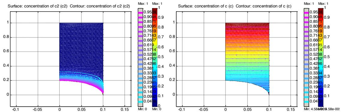
Figure 9 and 10: Concentration Profiles for Oxygen (c2) and the Electrolyte (c) for a Diffusivity Ratio = 0.8, Damkohler Number = 10
