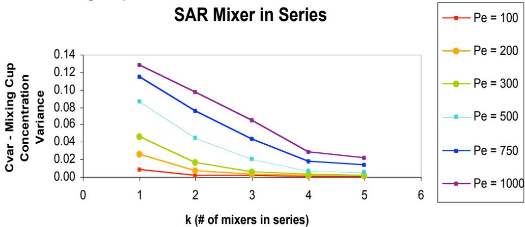
Figure 6: The change in the mixing cup concentration variance, over the number of mixers in series, is depicted above for six different Peclet number values to show six different values of flow.
