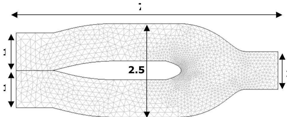
**Figure 3:** The two-dimensional model of the optimized SAR mixer as modeled in COMSOL Multiphysics 3.4, rotated by 90° counter clockwise. The minimum channel width is standardized to 1. From this view, the inlets are at the left-side and flow goes from left to right. The second level mesh is shown (Fine) with 2616 elements and 17579 degrees of freedom.
