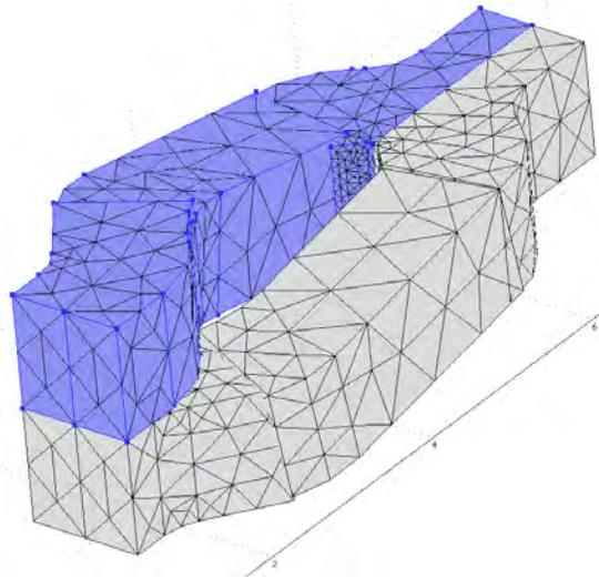
**Figure 8:** The expected 3D model in COMSOL is shown above using approximations with shapes. The two inlets are shown to the bottom left, where the stacked inlets (the split) is an important feature of the SAR mixer. The left side is highlighted in purple to show the separation between the two split streams and the top right represents the outlet, where both streams combine to a single channel.
