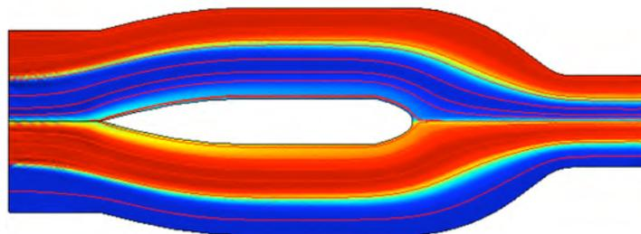
**Figure 4:** The solution to the two-dimensional model with the velocity streamlines and concentration surface plot is depicted above, rotated by 90° counter clockwise. The red represents a concentration of 1 whereas indigo is a concentration of 0, equal mixing is green with a value of 0.5, and the variation in color represents the concentration gradient. For a Peclet number of 1000 on Mesh #3 (10464 elements and 69615 degrees of freedom), the lamellae layers are clearly shown.
