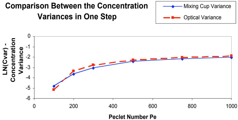
**Figure 8:** The change in the natural log of the mixing cup and optical concentration variances is plotted over varying Peclet numbers from 100 to 1000, representing changes in diffusivity.
