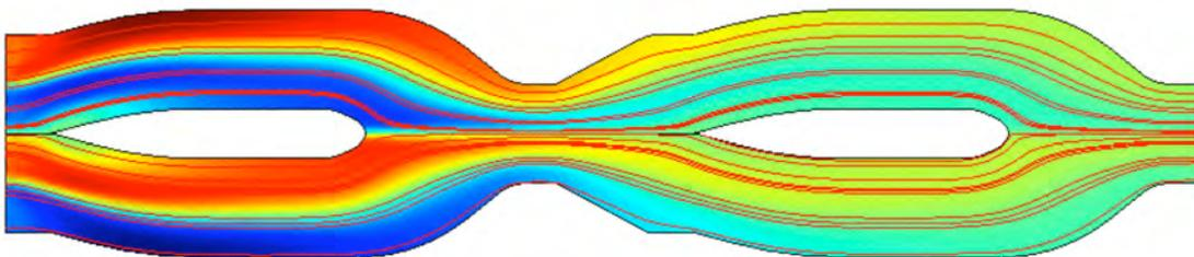
**Figure 5:** The solution for the two-dimensional model in a series of 2 is shown, rotated by  $90^\circ$  counter clockwise, for a Peclet number 1000 and on the third mesh (5236 elements, 35144 degrees of freedom).
