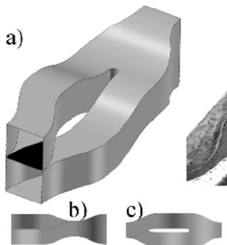
**Figure 2:** The optimized SAR mixer as introduced by Schönfeld et al. The overall geometry in 3D is shown in (a), whereas the side and top views are shown in (b) and (c) respectively. Source: Schönfeld, F. et al. “An optimized split-and-recombine micro-mixer with uniform ‘chaotic’ mixing.” *Lab Chip*, 2004, **4**, 65-69
