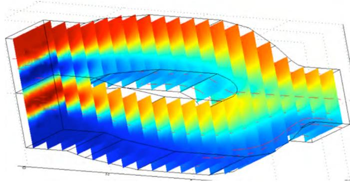
**Figure 9:** The 3D model used for concentration characterization is depicted, where the two inlets are to the left and the flow goes towards the right. The equivalent boundary conditions and subdomain settings are used for the walls, the inlets and the outlets of the geometry. The solution is shown for a Peclet number of 1000 and using the third mesh (30081 elements, 201852 degrees of freedom).
