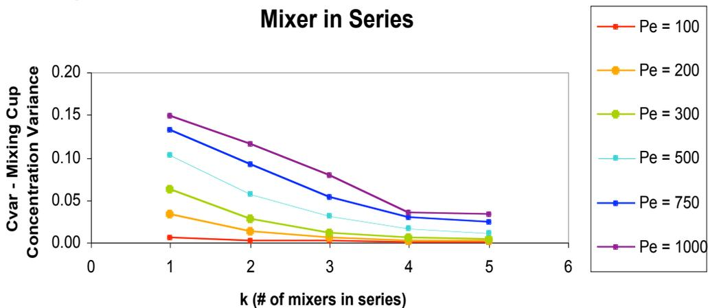
**Figure 7:** The change in the optical concentration variance, over the number of mixers in series, is depicted above for six different Peclet number values to show six different values of flow.
