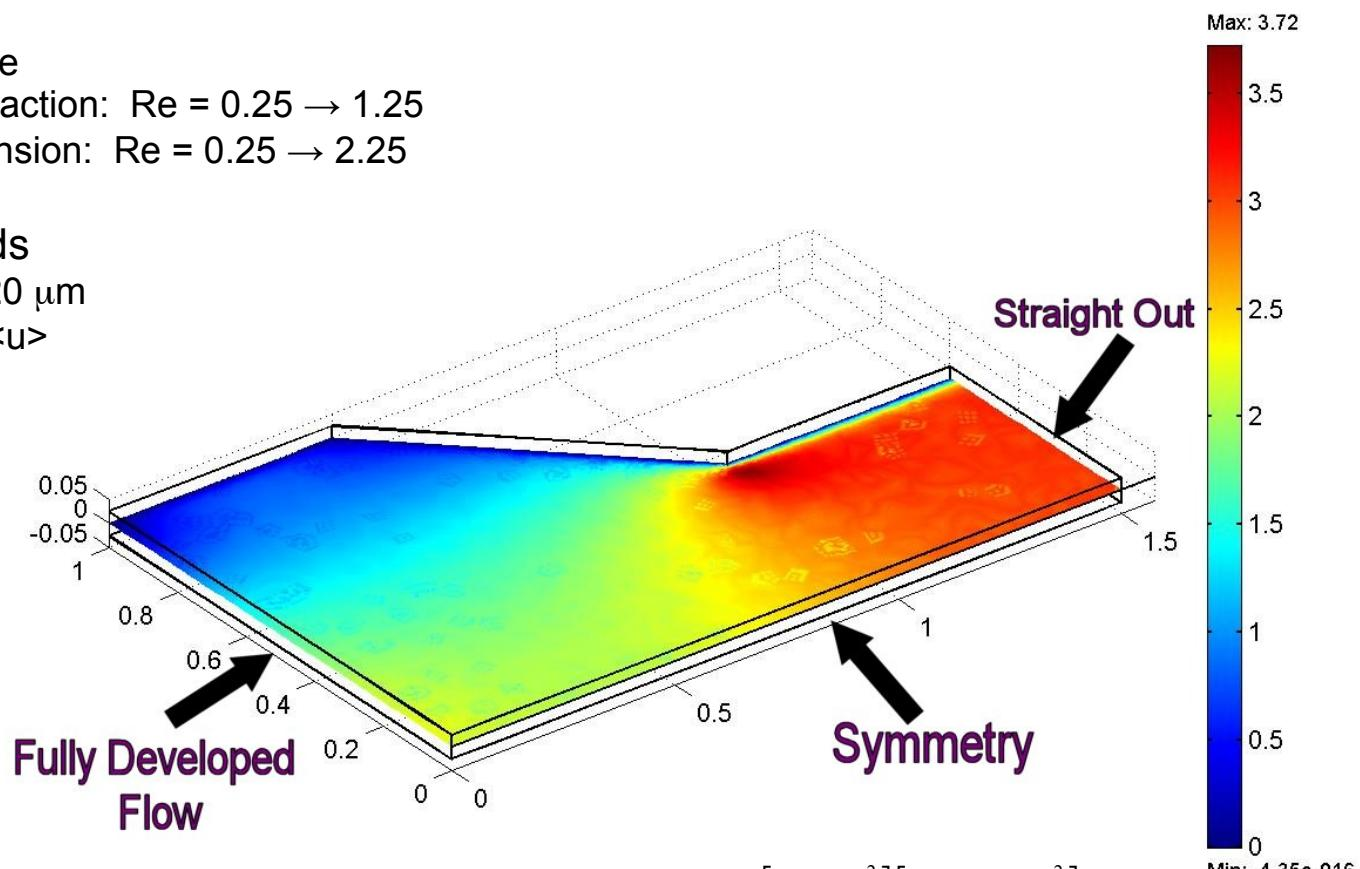
**Inlet Velocity Profile:**  $u(x) = \frac{9}{4} \left[ 1 - \left( \frac{y}{1} \right)^2 \right] \left[ 1 - \left( \frac{z}{0.025} \right)^2 \right]$
