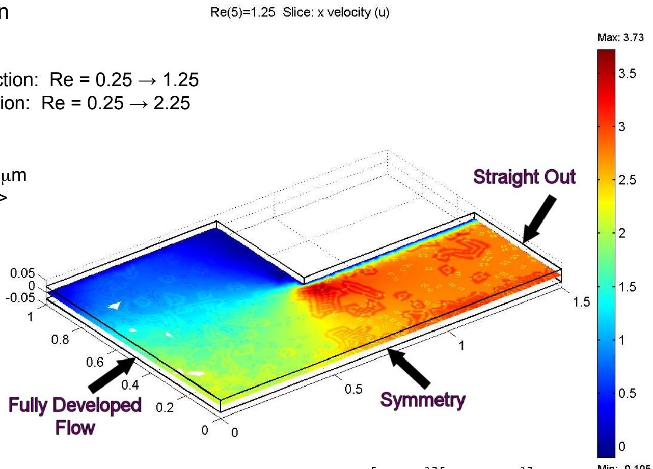
Inlet Velocity Profile:  $u(x) = \frac{9}{4} \left[ 1 - \left( \frac{y}{1} \right)^2 \right] \left[ 1 - \left( \frac{z}{0.025} \right)^2 \right]$
