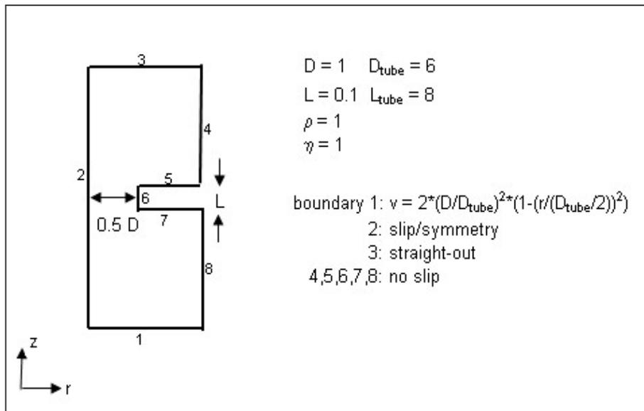
**Figure 5. The model and dimension used in FEMLAB simulation. To get various result at different L/D ratio, the orifice diameter (D) was kept constant while changing the orifice thickness (L). A fully developed flow was introduced at the entrance of the channel.**
