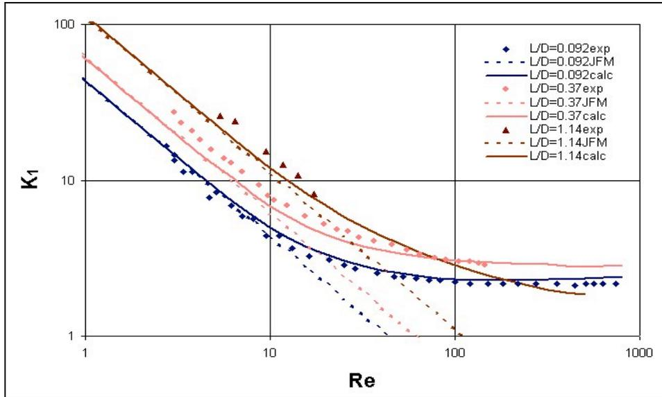
**Figure 9.** The results after the domain length was made longer to get fully developed velocity along the domain. Notice that at  $Re > 200$ , the domain should be made longer to get fully developed velocity along the domain.
