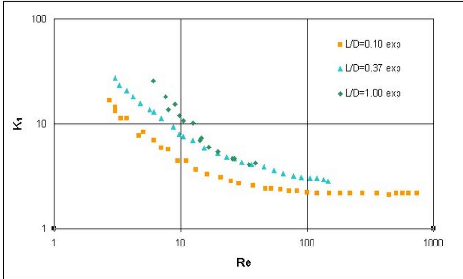
Figure 2. The experimental results taken from Hasegawa<sup>1</sup> for different L/D ratio. The experiment was done using water, silicon oils, and solutions of glycerin in water. This plot was reproduced from Hasegawa<sup>1</sup>.
