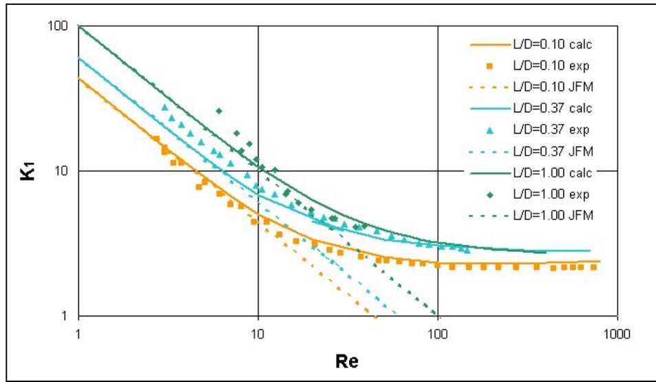
**Figure 6.** The dimensionless  $\Delta p$  ( $K_1$ ) from FEMLAB simulation was plotted against  $Re$  for different  $L/D$  ratio. At low  $Re$ ,  $K_1$  decreased as the increasing of  $Re$  and starts to level off at high  $Re$ .
