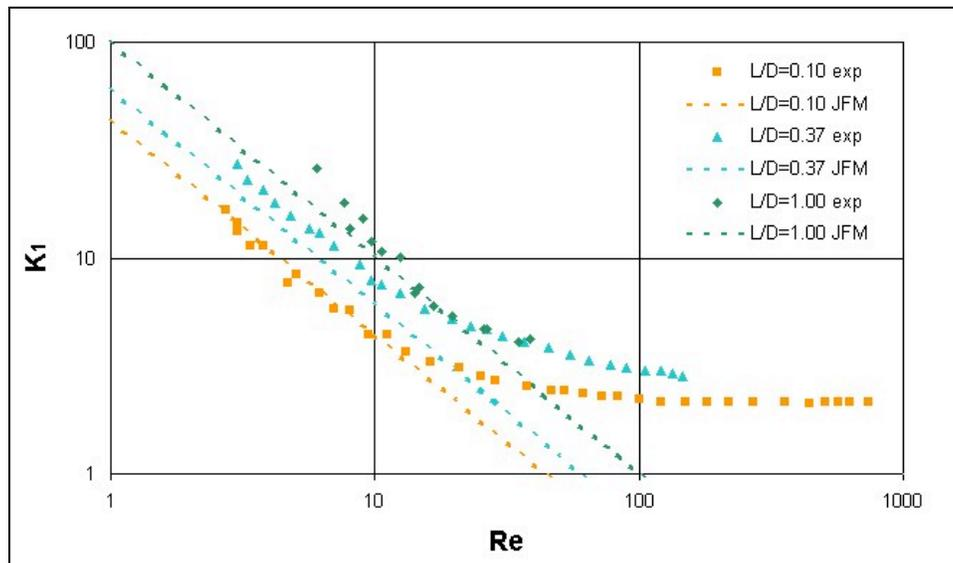
**Figure 4. The first evidence from analytical solution using exact solution slow flow. The equation used to get the analytical solution, called JFM, was taken from Dagan<sup>2</sup>.**
