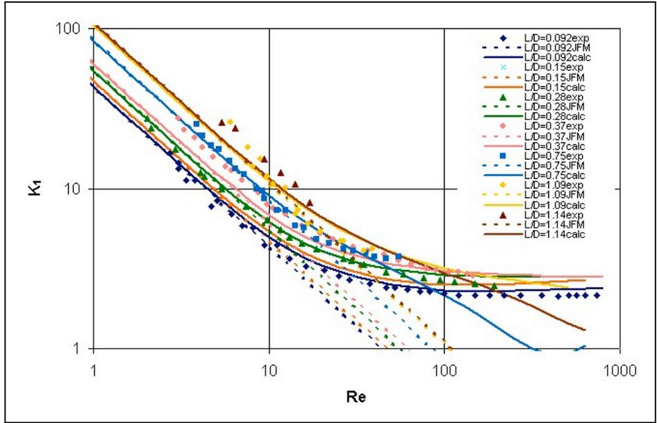
Figure 7. All results at different L/D ratio each for Hasegawa experiment result (exp, points), Dagan analytical solution (JFM, dotted line), and numerical solution using FEMLAB (calc, solid line). Note that at high Re, for high L/D ratio, the FEMLAB solution starts to deviate from what they supposed to be.
