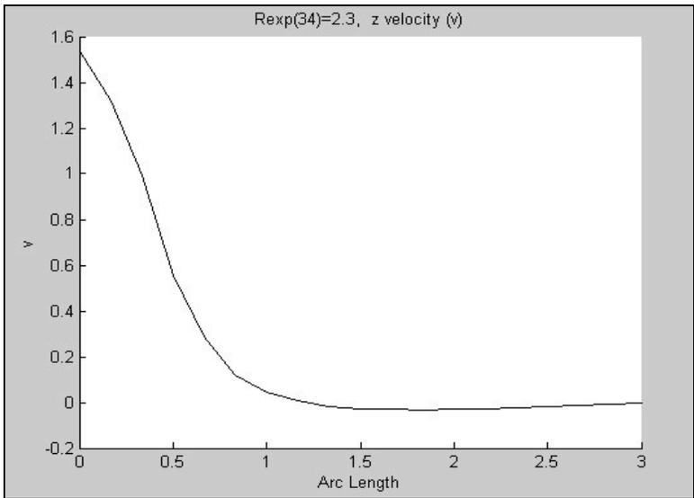
Figure 8. The exit velocity for L/D = 1.14 at Re = 200. It shows that the profile was not hyperbolic, means the velocity at the exit of the channel was not fully developed.
