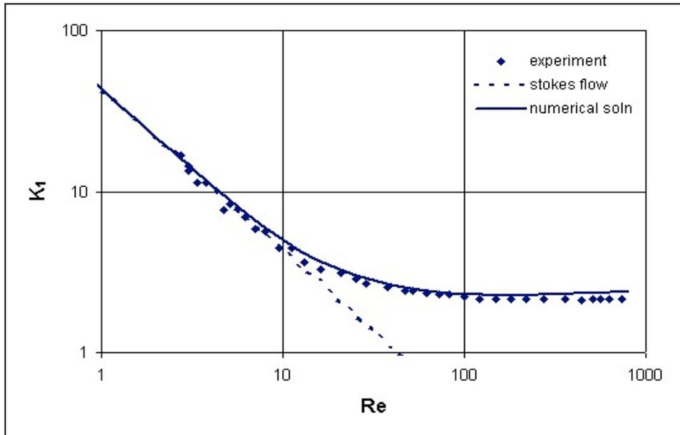
Figure 3. Numerical solution done by Hasegawa. Note here that they only have one numerical solution for different L/D ration. This plot was reproduced from Hasegawa<sup>1</sup>.
