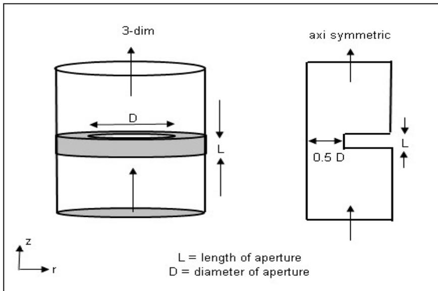
**Figure 1. The three dimensional orifice and the approximation using two dimensional, axisymmetric.**
