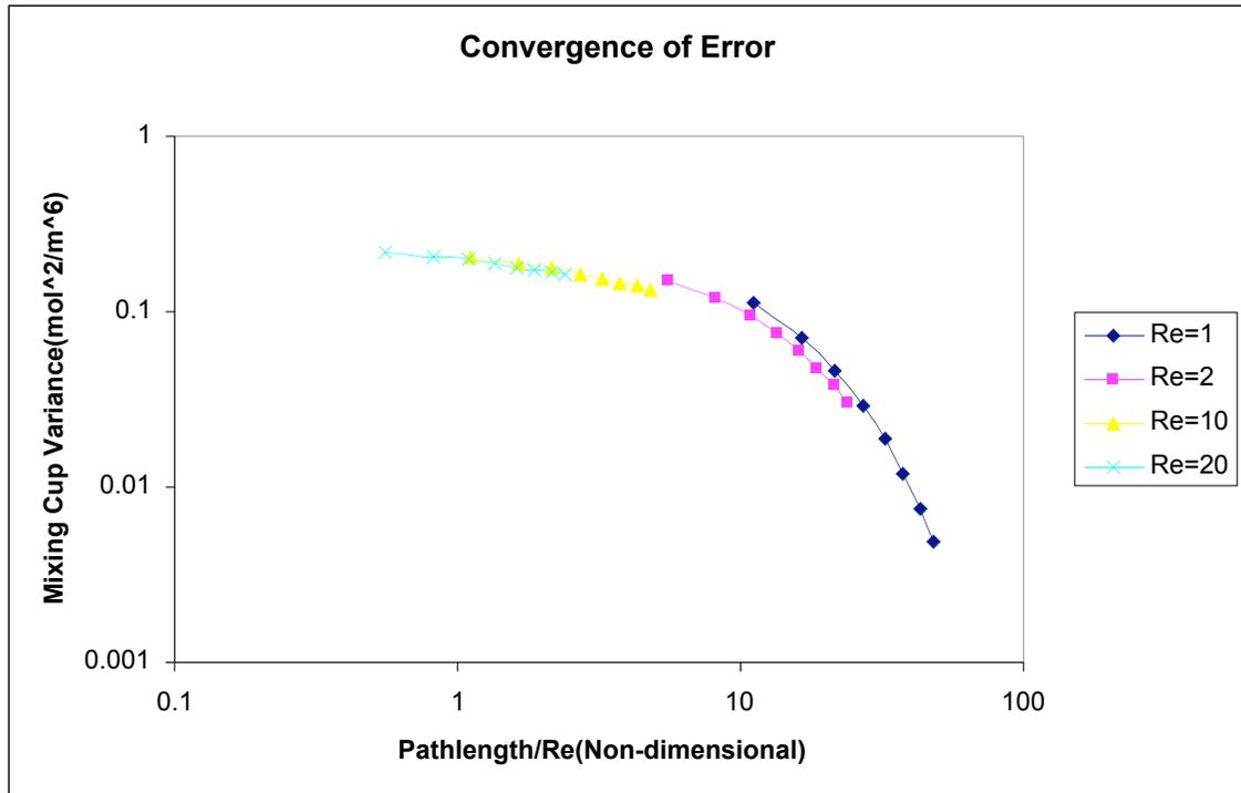
**Figure 4.** With the path-length in a ratio with the Reynolds number, the variances for varying Reynolds numbers converge to the same curve.
