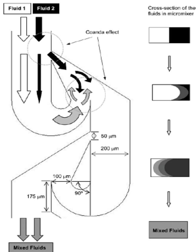
**Figure 1. Modified Tesla Mixer and Coanda Effect**
