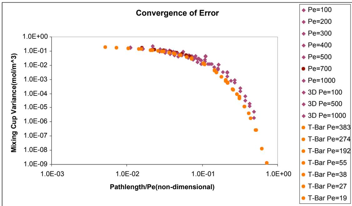
**Figure 7. Comparison of the evaluated Tesla mixer and a T-shaped mixer.**
