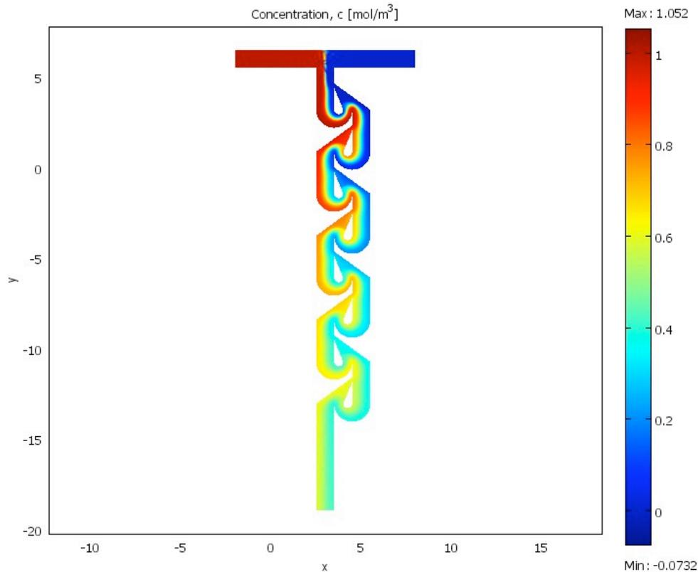
**Figure 2. Solution of Convection-Diffusion equation from Comsol.**
