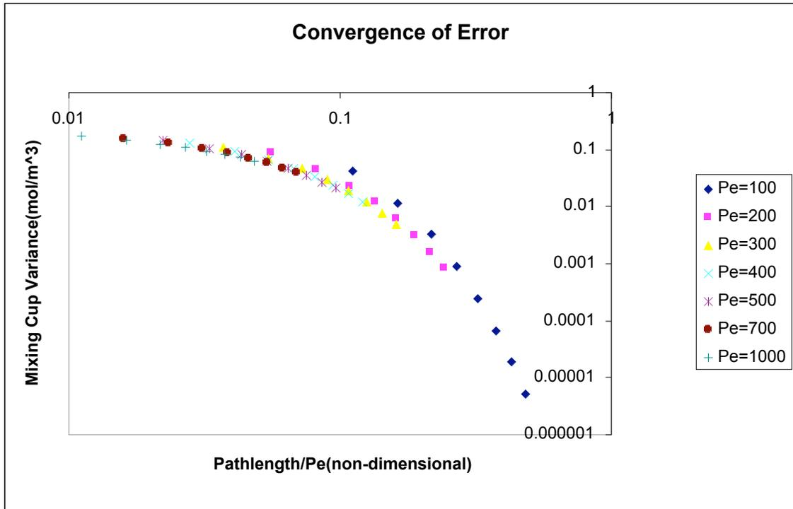
**Figure 3.** With the path-length in a ratio with the Peclet number, the variances for varying Peclet numbers converge to the same curve.
