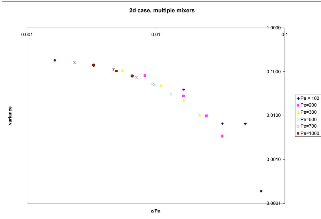
Figure 4. Log-log graph of the variance versus the characteristic length ( $z$ ) to Pe ratio. The variance increases with increasing Pe number, meaning that the variance decreases as the  $z/Pe$  ratio increases.
