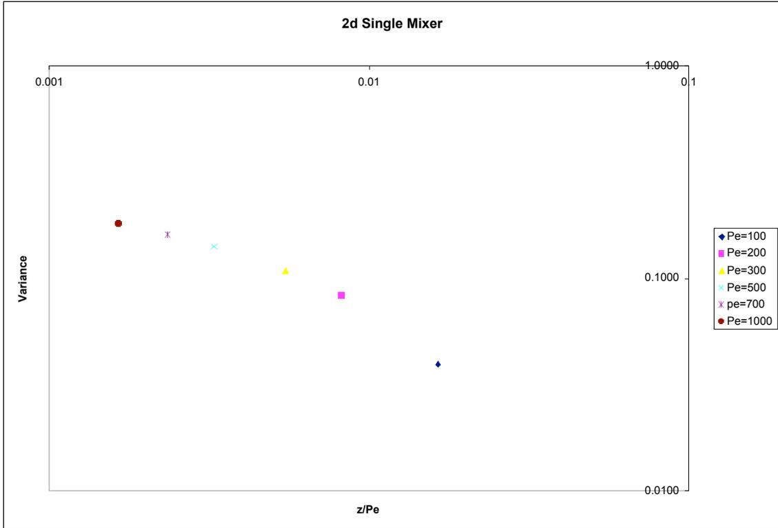
**Figure 6.** 2D mixer. Variance versus ratio of  $z/Pe$ .
