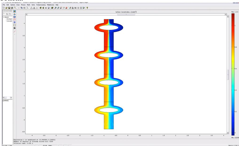
Figure 2. Comsol model for tear drop mixer. The concentration profile shown is for a Péclet of 500.
