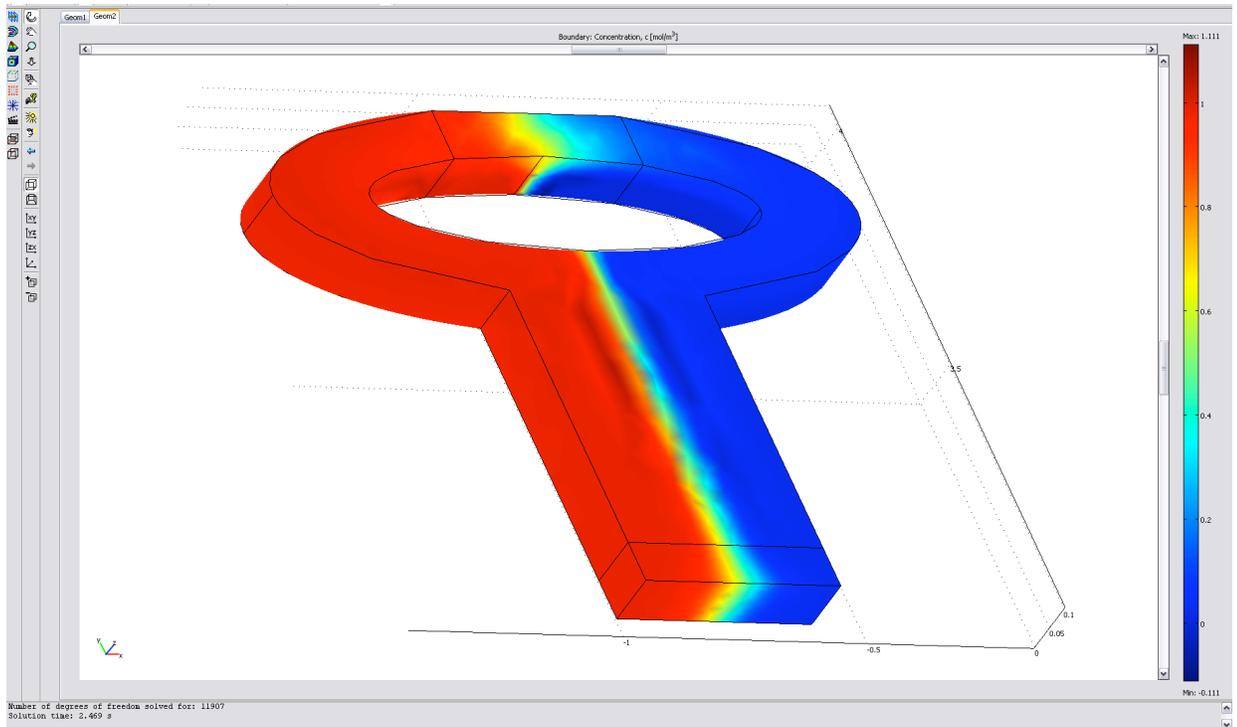
**Figure 3.** 3D shape in Comsol model. The concentration shown is for a Peclet number of 500.
