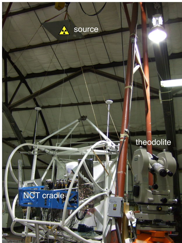
Figure 6.2: Laboratory setup for effective area calibrations.
