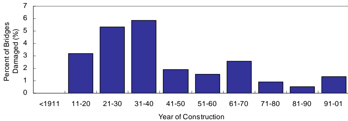
Figure 3.1. Effect of the year of construction on the percentage of damaged bridges.
