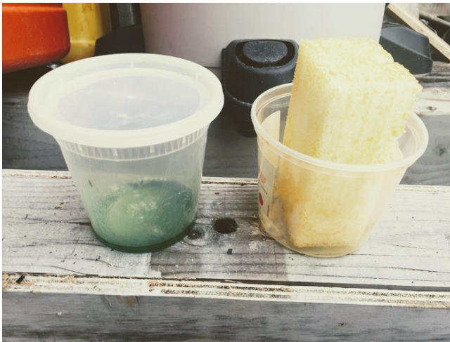
Figure 6: Senior UCD undergraduate and former chemistry major Betsy's packing foam experiments, which emerged from her concern for plastic pollution. She dissolved polystyrene packaging (L) into adhesive, string-like threads, and putty. She found other forms of foam (R) did not dissolve.
