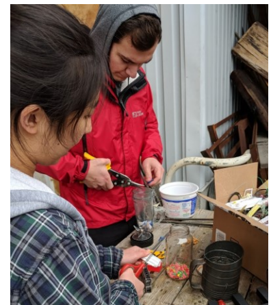
Figure 1: Student designers sort, clean, and mill PLA scraps from discarded 3D prints.
