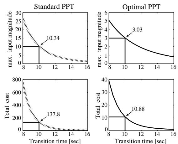
Fig. 6. Comparison of costs and maximum input magnitudes for standard PPT (dotted line) and optimal PPT (solid line) when the transition time  $T_{tran} = t_f - t_i$  is varied. It is noted that the cost for optimal PPT is always less than the cost for standard PPT.
