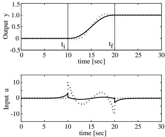
Fig. 4. Comparison of output and input time-trajectories for standard PPT (dotted line) and optimal PPT (solid line)—the optimal PPT input has pre- and post-actuation, however, the time for output transition is the same (10 s) for both methods. The output transition is initiated at time  $t = t_i = 10$  s and completed at time  $t = t_f = 20$  s.
