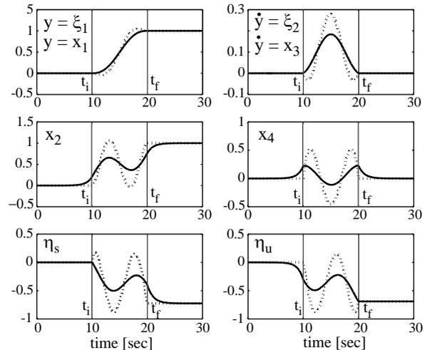
Fig. 5. Comparison of state time-trajectories for standard PPT (dotted line) and optimal PPT (solid line) with input weight  $R = 1$ . The stable and unstable components of the internal state ( $\eta_s$ , and  $\eta_u$ ) are shown in the bottom plots.
