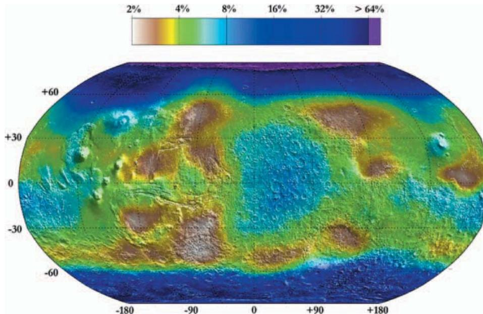
**FIGURE 1** Water-equivalent hydrogen content of subsurface water-bearing soils derived from the *Mars Odyssey* neutron spectrometer. (From Feldman et al., 2004, *J. Geophys. Res.* **109**, E09006, doi:10.1029/2003JE002160.)
