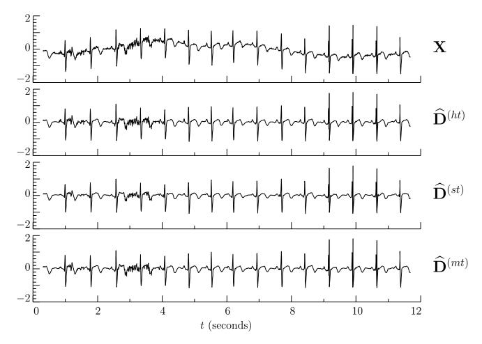
• hard/soft/mid threshold estimates with  $J_0 = 6$  partial LA(8) DWT, MAD & scaling coefficients to 0 (zaps baseline drift)
