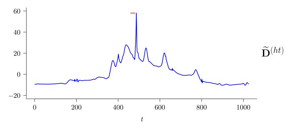
• signal estimate using  $J_0 = 6 \text{ LA}(8) \text{ MODWT}$  with hard thresholding
