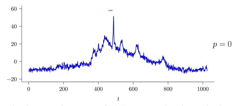
• shrinkage signal estimates of NMR spectrum based upon level  $J_0 = 6$  partial LA(8) DWT and conditional mean with p = 0 (with this choice of p, estimator collapses to minimum mean square estimator of ovehead XI-37)
