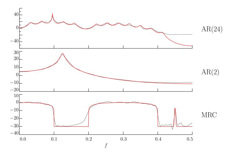
• SDF estimates (thin jagged) and true SDFs (thick smooth) for AR(24), AR(2) and mobile radio communications processes
