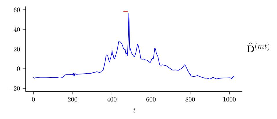
• signal estimate using  $J_0 = 6$  partial LA(8) DWT, but now with mid thresholding
