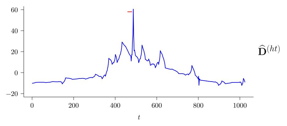
• signal estimate using  $J_0 = 6$  partial D(4) DWT with hard thresholding and universal threshold level estimated by  $\hat{\delta}^{(u)} = \sqrt{[2\hat{\sigma}_{(\text{mad})}^2 \log(N)]} \doteq 6.49$
