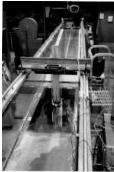
Figure 4.4: View over the tank, the cylinder above the plexiglas window can be seen in the center of the picture
