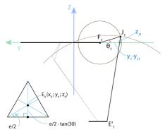
▶  $E_1$  is the projection of  $E_0$  to the bottom side of the end effector triangle on the XZ plane:
