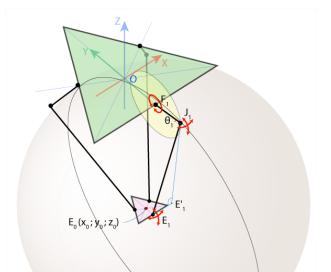
► The sphere intersects with the YZ plane, forming a circle with center  $E'_1$  and radius  $E'_1J_1$ :
