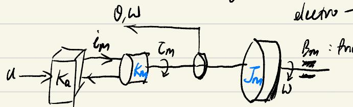
motor driver      motor      encoder      motor inertia
