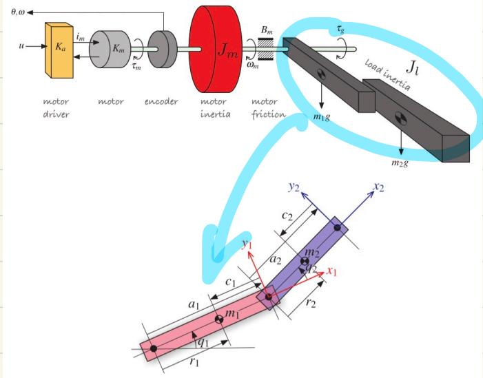
torque acting on joint 1: (from dynamics)
