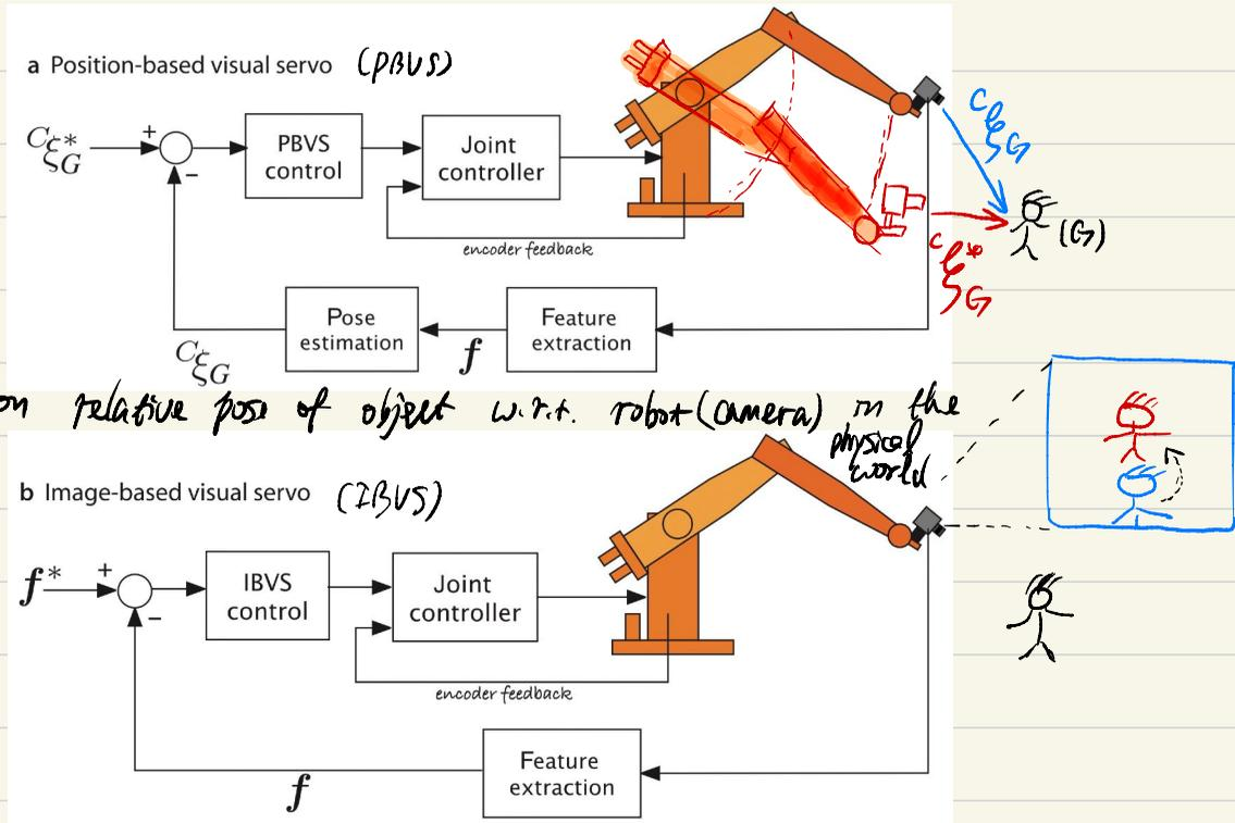
PBVS: focus on relative pose of object w.r.t. robot (camera) in the physical world
