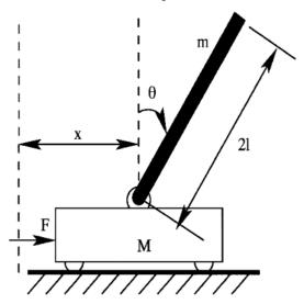
The mass of the cart is  $m_c$ , the mass and moment of inertia (about mass center) of the pendulum are  $m_p$ ,  $I_p$  respectively. The pendulum is attached to the cart at a frictionless pivot point. The pendulum's center of mass is l units from the pivot. The coordinate x measures the position of the cart (a point-mass) relative to an inertial frame. F is an applied external horizontal force to the cart.
