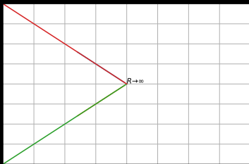
Figure: Eigenvalue \lambda_{1,2} = -\frac{1}{\sqrt{2R^{1/4}}} \pm \frac{1}{\sqrt{2R^{1/4}}}j evolution (root locus)
