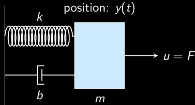
$$\begin{aligned}\underbrace{\frac{d}{dt} \begin{bmatrix} y(t) \\ v(t) \end{bmatrix}}_{x(t)} &= \underbrace{\begin{bmatrix} 0 & 1 \\ -\frac{k}{m} & -\frac{b}{m} \end{bmatrix}}_A \underbrace{\begin{bmatrix} y(t) \\ v(t) \end{bmatrix}}_{x(t)} + \underbrace{\begin{bmatrix} 0 \\ \frac{1}{m} \end{bmatrix}}_B u(t) \\ y(t) &= \underbrace{\begin{bmatrix} 1 & 0 \end{bmatrix}}_C \underbrace{\begin{bmatrix} y(t) \\ v(t) \end{bmatrix}}_{x(t)}\end{aligned}$$
