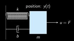
$$\frac{\frac{d}{dt}}{\underbrace{\begin{bmatrix} p(t) \\ v(t) \end{bmatrix}}} = \underbrace{\begin{bmatrix} 0 & 1 \\ -\frac{k}{m} & -\frac{b}{m} \end{bmatrix}}_{A} \underbrace{\begin{bmatrix} p(t) \\ v(t) \end{bmatrix}}_{x(t)} + \underbrace{\begin{bmatrix} 0 \\ \frac{1}{m} \end{bmatrix}}_{B} u(t)$$
