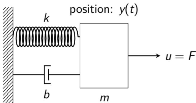
$$\underbrace{\frac{d}{dt} \begin{bmatrix} y(t) \\ v(t) \end{bmatrix}}_{x(t)} = \underbrace{\begin{bmatrix} 0 & 1 \\ -\frac{k}{m} & -\frac{b}{m} \end{bmatrix}}_A \underbrace{\begin{bmatrix} y(t) \\ v(t) \end{bmatrix}}_{x(t)} + \underbrace{\begin{bmatrix} 0 \\ \frac{1}{m} \end{bmatrix}}_B u(t)$$
