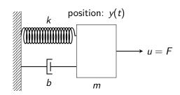
$$\frac{\frac{d}{dt} \underbrace{\begin{bmatrix} y(t) \\ v(t) \end{bmatrix}}_{x(t)} = \underbrace{\begin{bmatrix} 0 & 1 \\ -\frac{k}{m} & -\frac{b}{m} \end{bmatrix}}_{A} \underbrace{\begin{bmatrix} y(t) \\ v(t) \end{bmatrix}}_{x(t)} + \underbrace{\begin{bmatrix} 0 \\ \frac{1}{m} \end{bmatrix}}_{B} u(t)$$
