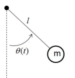
Input:  $u(t) = T_c(t)$ , torque to the pivot point
