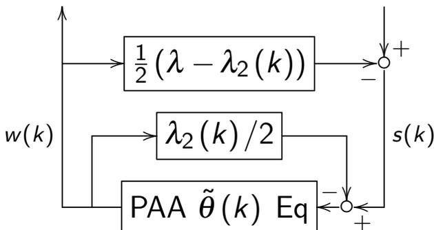
note that it is a feedback connection of a passive block with  $\frac{1}{2}(\lambda - \lambda_2(k)) \geq 0$
