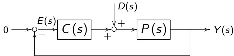
the “structure” of the reference/disturbance is built into the integral controller:
