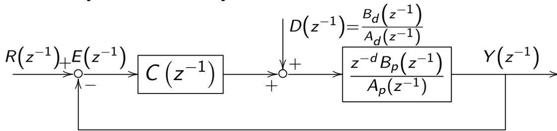
$$C(z^{-1}) = \frac{k_r z^{-N+\mu} A_p(z^{-1}) B_p^-(z) z^{-\mu}}{(1 - z^{-N}) B_p^+(z^{-1}) z^{-d} b}, \quad b > \max_{\omega \in [0, \pi]} |B_p^-(e^{j\omega})|^2 \quad (3)$$
