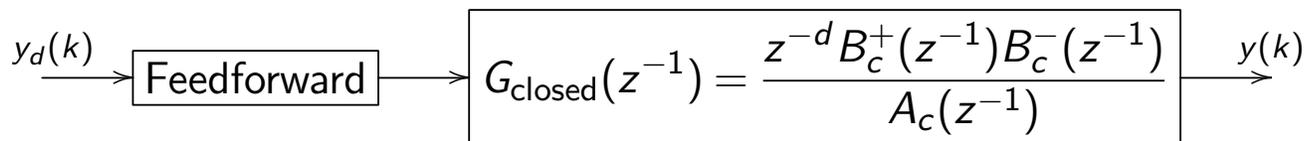
Zero Phase Error Tracking (ZPET): extend (3) by adding a  $B_c^-(z)$  part
