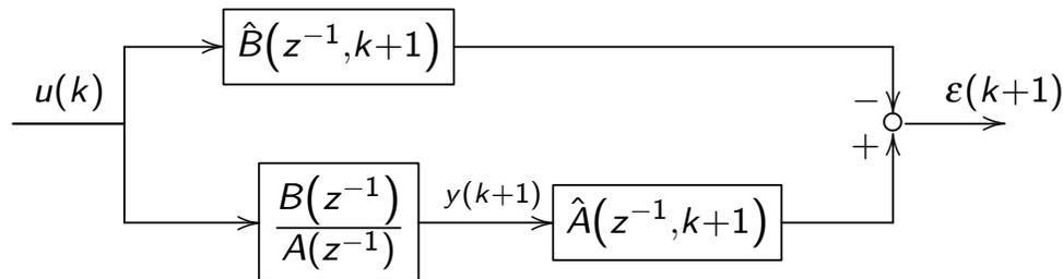
A series-parallel structure:  $\hat{A}(z^{-1}, k+1)$ —in series with plant;
