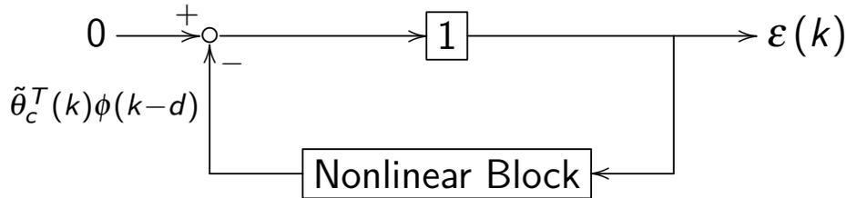
The PAA thus is in a standard series-parallel structure with the LTI block being 1. Hyperstability easily follows, which gives
