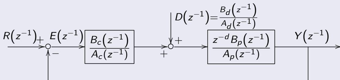
Assume  $B_p(z^{-1}) = 0$  and  $A_d(z^{-1}) = 0$  do not have common zeros. If the closed loop is asymptotically stable, and  $A_c(z^{-1})$  can be factorized as  $A_c(z^{-1}) = A_d(z^{-1})A'_c(z^{-1})$ , then the disturbance is asymptotically rejected.
