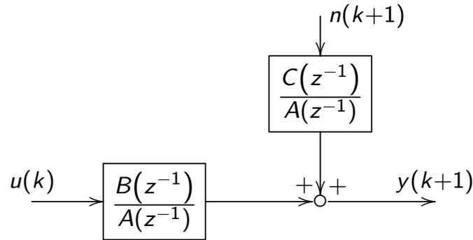
$$\text{i.e. } w(k+1) = C(z^{-1})n(k+1) = [1 + c_1z^{-1} + \dots + c_{n_C}z^{-n_C}]n(k+1)$$
