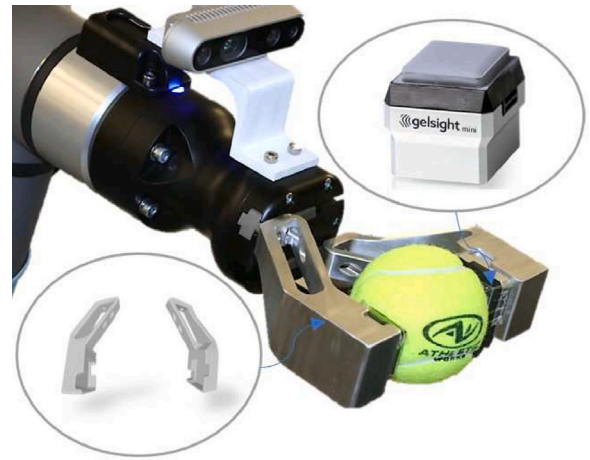
Fig. 2. Design of adapter for housing Gelsight tactile sensors. A 45-degree flange extension was designed for the end-effector to extend the opening distance of the gripper to 85 mm. The adapters are mounted on the Robotiq Hand-e adaptive gripper through four M2.5 screws.
