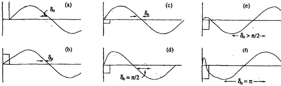
**Figure B-2:** Radial wave functions for low-energy, *s*-wave scattering by a square well. For comparison, the corresponding form for a free particle is shown as a dotted curve in each case. The result of an infinite repulsive well is shown in (a) and a finite one in (b). The results for attractive potentials of different depths are shown in (c) to (f). The wave functions inside the well in these cases grow faster near the origin than that for a free particle and the phase shift is positive.
