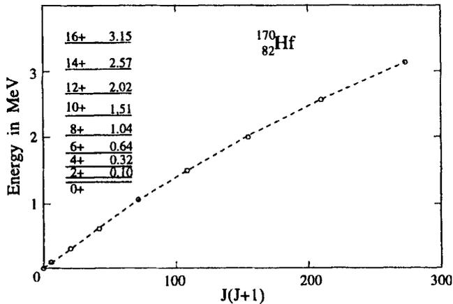
**Figure 6-10:** Rotational levels in  $^{170}\text{Hf}$ . For a simple rotor, the relation between  $E_J$  and  $J(J + 1)$  is a curve with constant slope. The small curvature found in the plot indicates that  $\mathcal{I}$  increases slightly with large  $J$ , a result of centrifugal stretching of the nucleus with increasing angular velocity. (Plotted using data from Ref. [95].)
