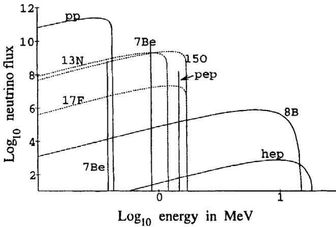
**Figure 10-5:** Log-log plot of the expected neutrino fluxes from various proton burning reactions in the sun [19]. Solid curves are those from PP-chains and dotted curves from the CNO cycle. Discrete lines come from a *pep* reaction and  ${}^7\text{Be}$  from electron capture.
