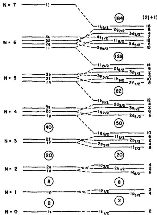
Figure 7-3: Schematic diagram of single-particle energy spectrum for spherical shell model. The lowest three major shells, 1s, 1p and 2s1d, are the same as those produced by a three-dimensional, isotropic harmonic oscillator well. The higher major shells include also the orbit with the largest j-values lowered in energy from the harmonic oscillator shell above by spin-orbit energy.
