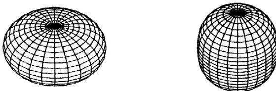
**Figure 6-9:** Quadrupole-deformed shapes for axially symmetric nuclei. On the left, the oblate shape has  $\beta = -0.4$ , and on the right, the prolate shape has  $\beta = +0.4$ .
