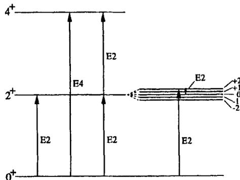
**Figure 8-2:** Low-lying energy level spectrum of a hypothetical even-even nucleus showing first-order and second-order Coulomb excitation processes.
