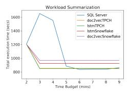
Figure 3: Workload runtime using indexes recommended under various time budgets. For most time budgets, the workload summaries improve runtimes, even when the embedders were trained on an unrelated workload (lstm-Snowflake and doc2vecSnowflake).
