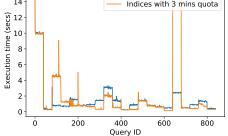
Figure 4: Runtime for each query under no indexes and under indexes recommended with a three-minute time budget. For a few specific queries, the presence of a recommended index results in significantly worse performance.
