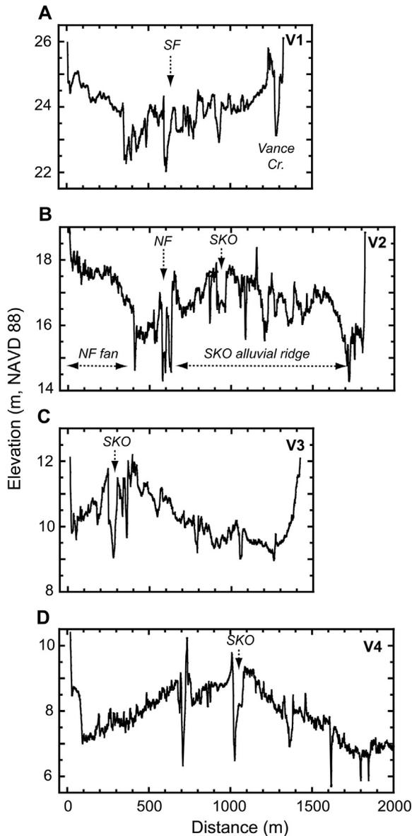
**Fig. 5.** Topographic profiles, from water-penetrating 2015 lidar, across the Skokomish River valley at four representative locations shown in Fig. 4. Profiles are from left to right, looking down valley (north to south). Labels and arrows are locations of the channels of the South Fork Skokomish (“SF”), North Fork (“NF”), Skokomish (“SKO”), and Vance Creek.
