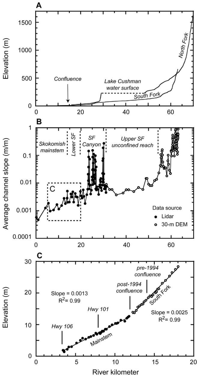
**Fig. 3.** (A) Longitudinal profile of the Skokomish River and forks, from 30-m digital elevation model (DEM). (B) Channel slope of the Skokomish and South Fork Skokomish rivers, from lidar and 30-m DEM. (C) Slope of the Skokomish River mainstem and lower South Fork Skokomish River, from average bed elevations measured by cross sections surveyed in 2007.
