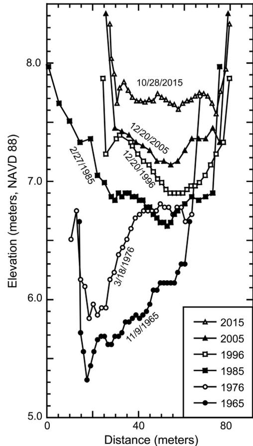
**Fig. 12.** Stream-bed elevation from gauging records at USGS gauge 12061500, Skokomish River near Potlatch, WA, 1965–2015. Representative cross sections are shown at approximately 10-yr intervals; discharge at selected cross sections ranged from  $30.0 \text{ m}^3 \text{ s}^{-1}$  ( $1060 \text{ ft}^3 \text{ s}^{-1}$ ) to  $126 \text{ m}^3 \text{ s}^{-1}$  ( $4440 \text{ ft}^3 \text{ s}^{-1}$ ).
