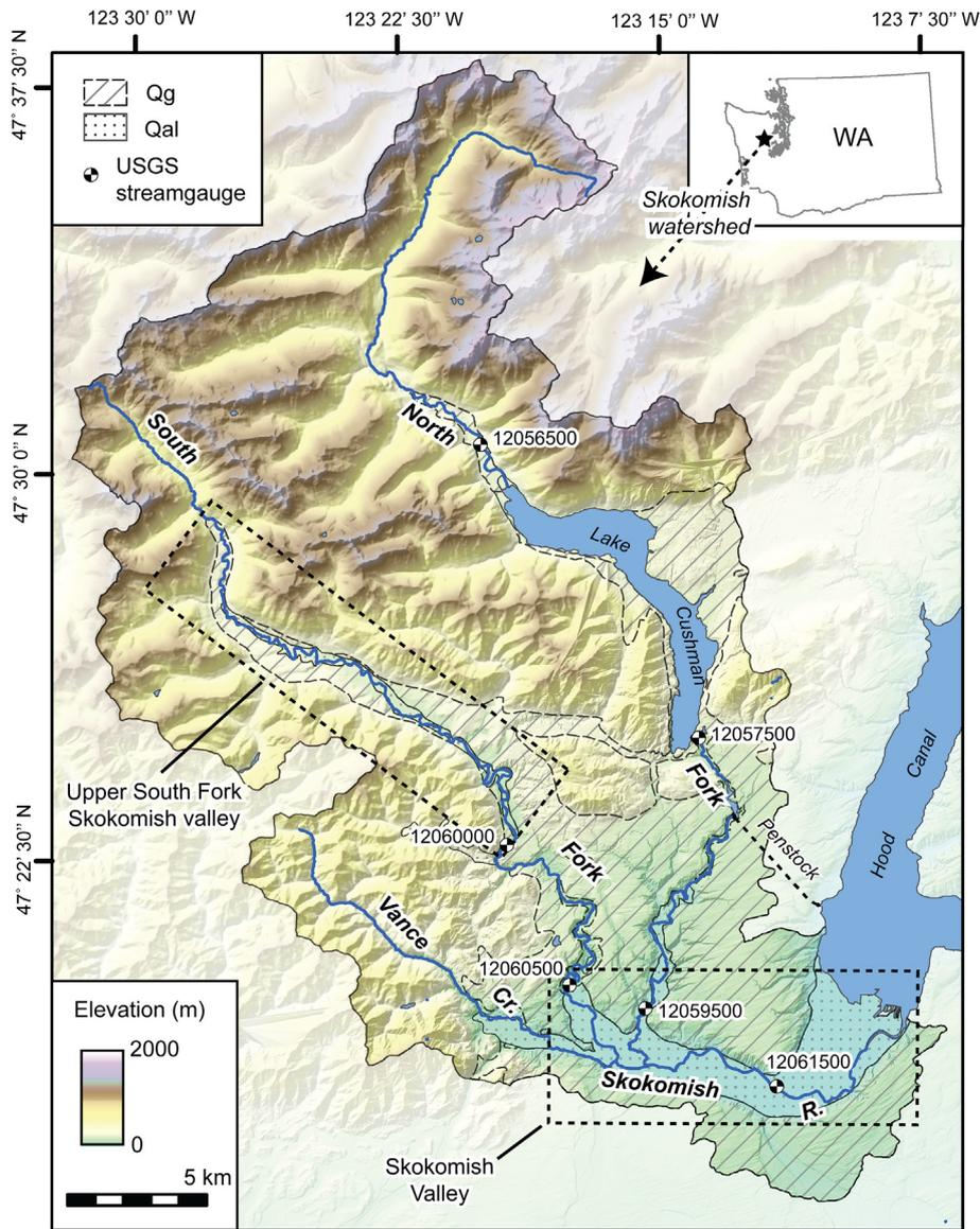
**Fig. 1.** Topography of the Skokomish River watershed in Washington State. Hatching shows extent of Pleistocene glacial drift (Qg) and stippled pattern shows Holocene alluvium (Qal), generalized from Logan (2003).
