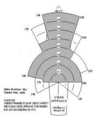
Figure 2. Ship-rotorcraft operational envelope
