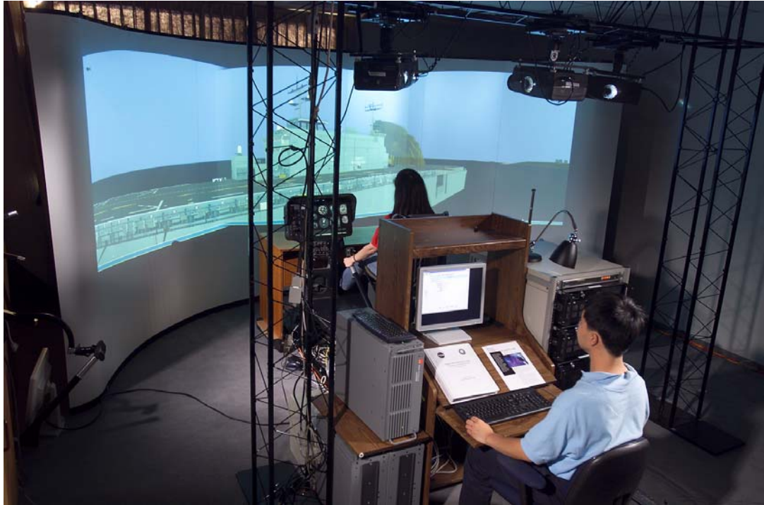
Figure 70. ART flight simulator with pilot in front of projection screen and operator at rear console
