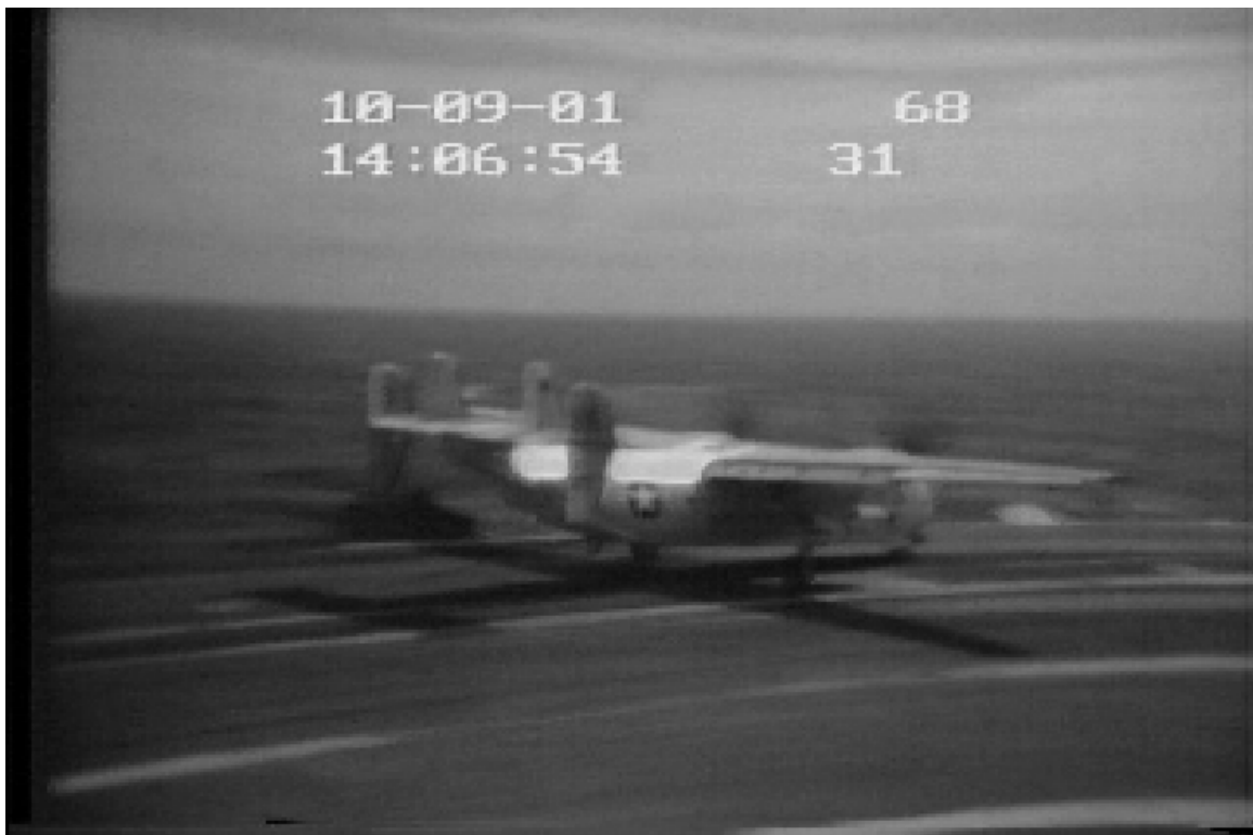
Figure 15. Aircraft landing gear slips off deck edge because pilot cannot compensate for crosswind
