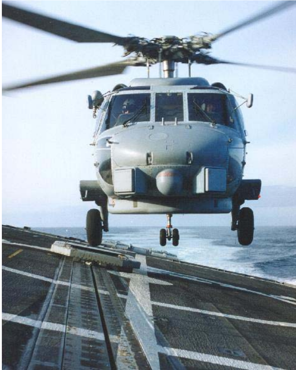
Figure 19. Helicopters landing on shipboard have to contend with high levels of pitch and roll (photo by K. Long, US Govt. image, courtesy of K. Long)
