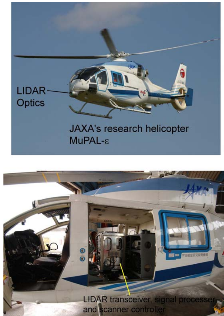
Figure 48. A helicopter-mounted lidar system undergoing test flights at the Japan Aerospace Exploration Agency (photo courtesy of Naoki Matayoshi)
