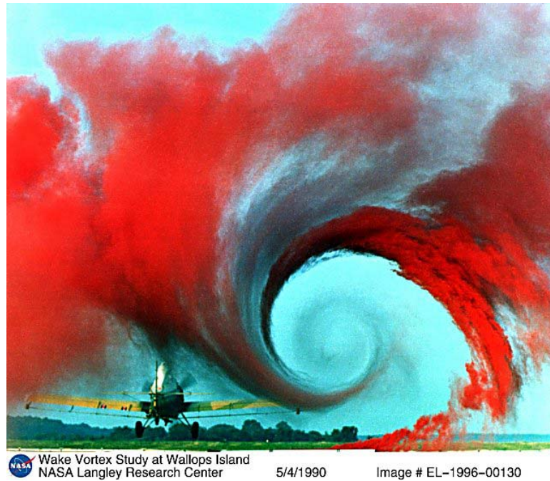
Figure 38. Example of experimental flow visualization - Wake vortex visualized by smoke and color enhancement (US Govt. image, http://www.larc.nasa.gov )
