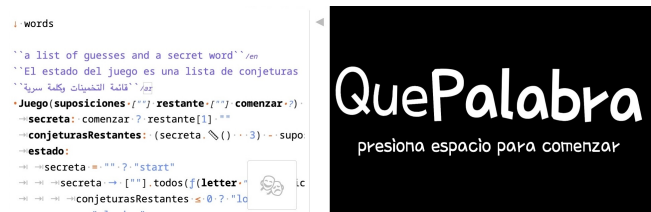
Figure 10: Programs can be rendered in one or more particular locales or with a preference for symbolic names. Here, a program is shown in Spanish, except for the comment the cursor is in.
