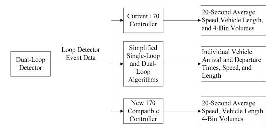
Figure 3. Data flow diagram for proposed research approach
