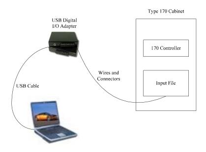
Figure 1. Overview of the laptop-based DEDAC system design
